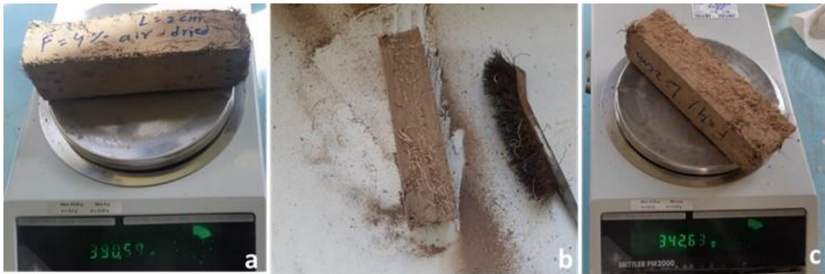
Figure 4. 27. Abrasion testing of earth bricks
