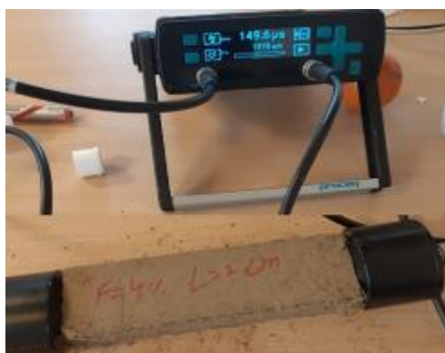
Figure 4. 21. Ultrasonic pulse velocity test set up
