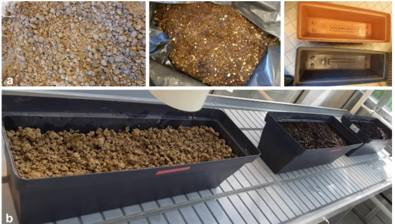
Figure 5. 8. Sediments - potting soil mixing (a) and pots filled with soil mixtures (b)
