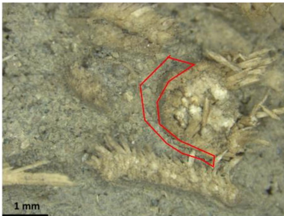
Figure 5. 32. Micro cracks development around hemp shiv.
