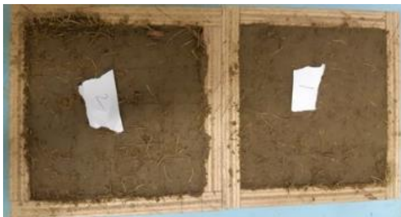
Figure 4. 25. Sample preparation for thermal conductivity test
