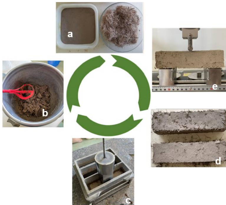
Figure 4. 19. Earth bricks manufacturing process
