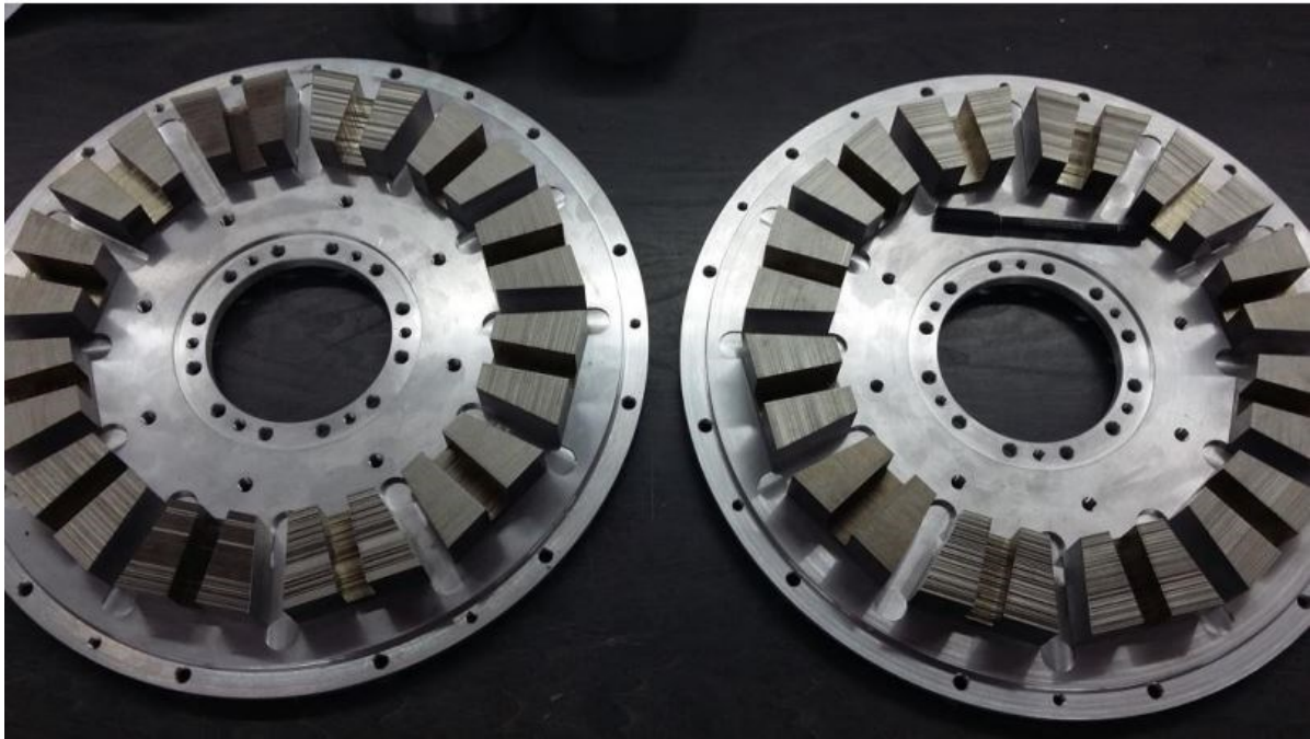
Fig. 1.39: Stator of the flux switching machine without magnets
