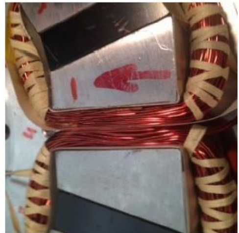
Fig. 1.40: Winding of the flux switching machine
