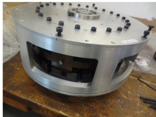
Fig. 1.42: Assembled flux switching machine
