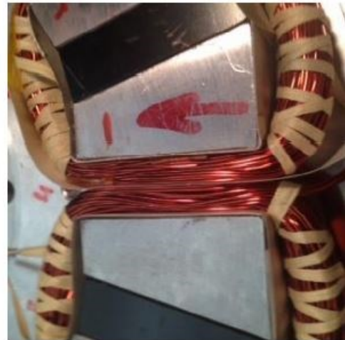
Fig. 1.40: Winding of the flux switching machine
