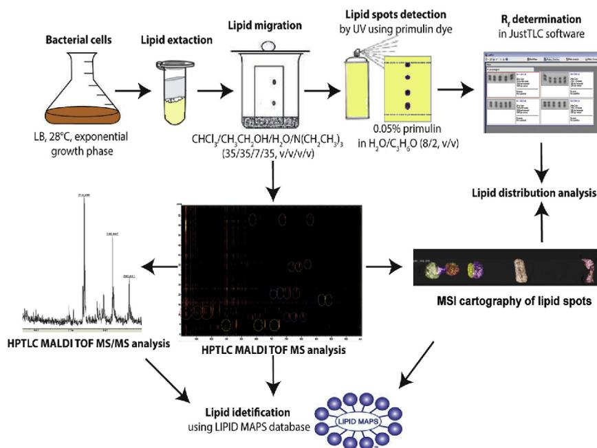
Fig. 1. Scheme illustrating the general HPTLC-MALDI TOF MSI method of PL class analysis.
