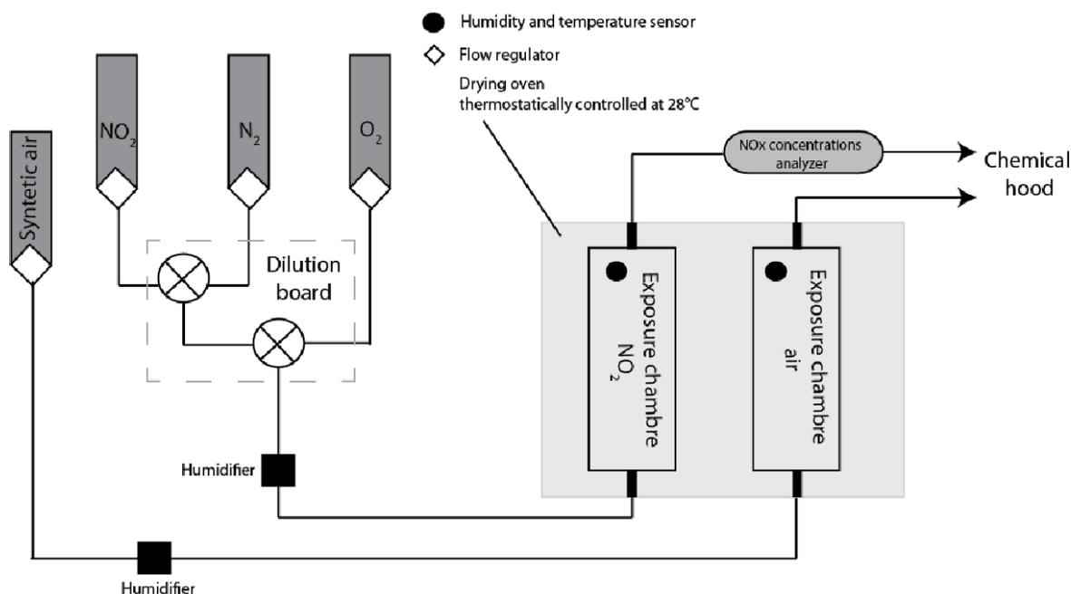
**Figure 1. Schematic representation of NO<sub>2</sub> gas delivery system**
