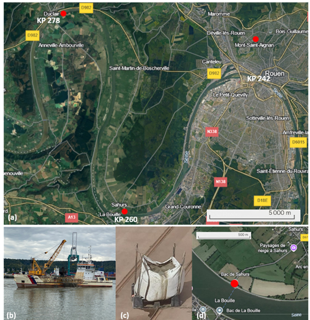
Figure 1. Sediment dredging on River Seine downstream of Port of Rouen: (a) Dredging location between KP 260 and KP278, (b) Dredger “Gambe d’Amfard” on River Seine; (c) Sediment big-bag container on the quay at La Bouille; (d) Location for agricultural spreading near Sahurs village.
