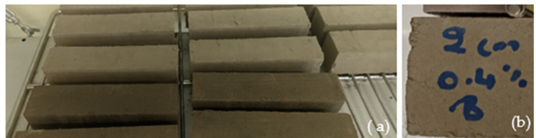
Figure 8. Sediment-based bricks: (a) during air drying at room temperature. Dark-colored bricks are just removed from the mold after manufacturing; the more they become dry, the more they are grey; (b) example of sample labelling: brick with 0.4% of fibers 2 cm long, sample B.
