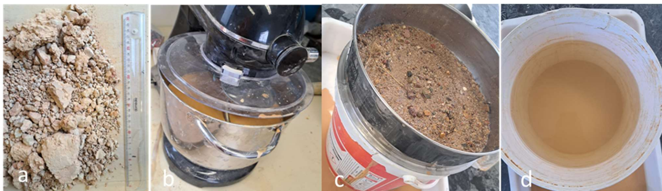
Figure 3. Raw soil (a), mixing soil with water (b), wet sieving of soil (c) and fine particles of soil (d).
