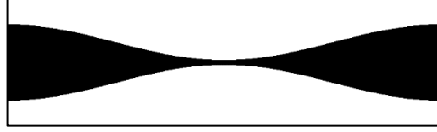
Figure 5: Synthetic image of a sinusoidally perturbed cylinder (unperturbed diameter: 70 pixels; image width and perturbation wavelength: 800 pixels; perturbation amplitude: 31 pixels)
