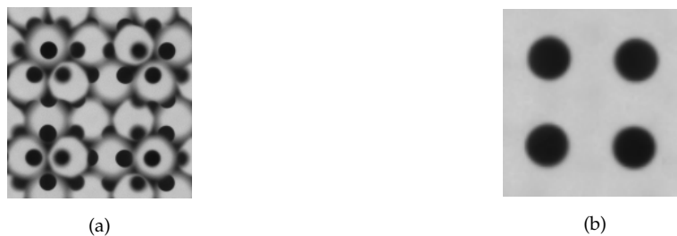
Figure 3. (a) Crop of a raw light field image of a calibration target, (b) Rendered all-focused image of the target
