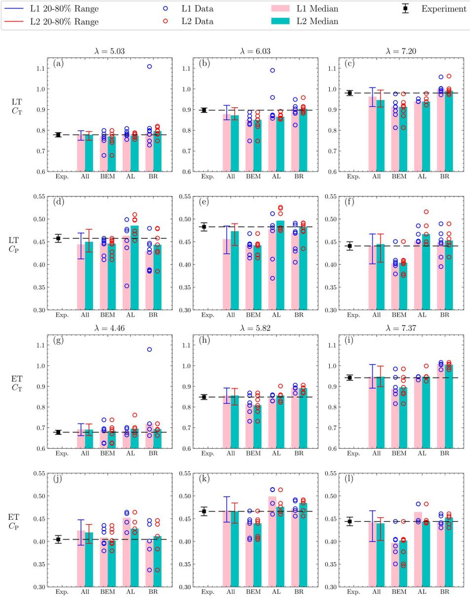
Fig. 4: Medians and ranges of integrated quantities,  $C_T$  and  $C_P$ , submitted as fully blind (L1) and user-error-corrected (L2) data for Low (LT) and Elevated (ET) turbulence levels. Three tip-speed ratios are shown at, above, and below the design operating point. The vertical bars indicate the 20-80% data range when considering all submissions, whilst the scatter dots are the submission values when considering submission by methodology.
