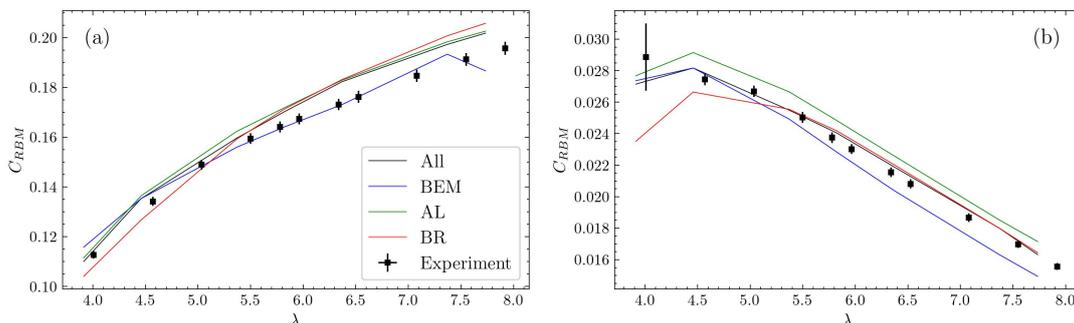
Fig. 6: Root bending moment coefficients,  $C_{RBM}$ , in flapwise (a) and edgewise (b) directions plotted by simulation method (median values) together with experiments for the elevated turbulence case.
