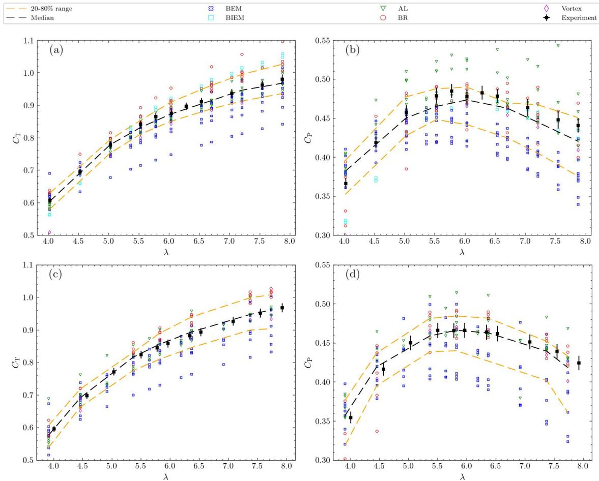
Fig. 3: Thrust and power coefficients,  $C_T$  and  $C_P$ , for the Low (a-b) and Elevated (c-d) turbulence cases. Experimental data are shown with a 95% confidence level, together with all blind simulation submissions. Submissions are categorised according to modelling techniques, and the median, 50%, and 20-80% data range of all submissions are indicated using dashed lines.
