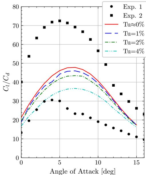
Fig. 2: Hydrofoil lift-to-drag ratios at turbulence intensity ( $Tu$ ) levels from 0.1% to 4% simulated using 2D RANS with  $k-\omega$  SST turbulence closure ( $Re = 2.88 \times 10^5$ ), and comparisons to experimental data; Exp. 1 at  $Re = 3.2 \times 10^5$  [9] and Exp. 2 at  $Re = 1.6 \times 10^6$  [10].
