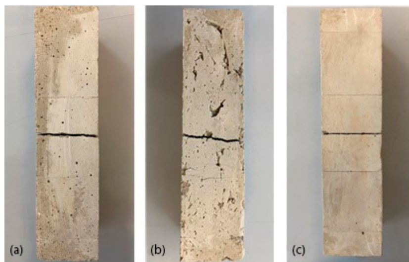
Figure 9. Flexural failure in (a) normalised mortar; (b) C s 1; (c) SG s 3.
