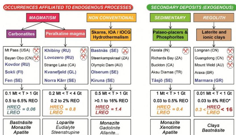
Figure 1.9. Characteristics of the main deposit models
