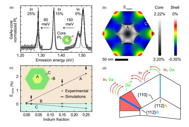
FIG. 3. (a) GaAs PL of NWs with In shell fraction of 0%, 15%, and 25%, acquired at 12 K with excitation laser of wavelength of 532 nm and power density of 100 W/cm<sup>2</sup>. (b) Hydrostatic strain simulation in core-shell NWs (25% In) as in Ref. [37]. (c) Simulated and average experimental ( $1\sigma$  error bar) hydrostatic strain vs In fraction. (d) Sketch of the Ga and In diffusion on the NW sidewalls.
