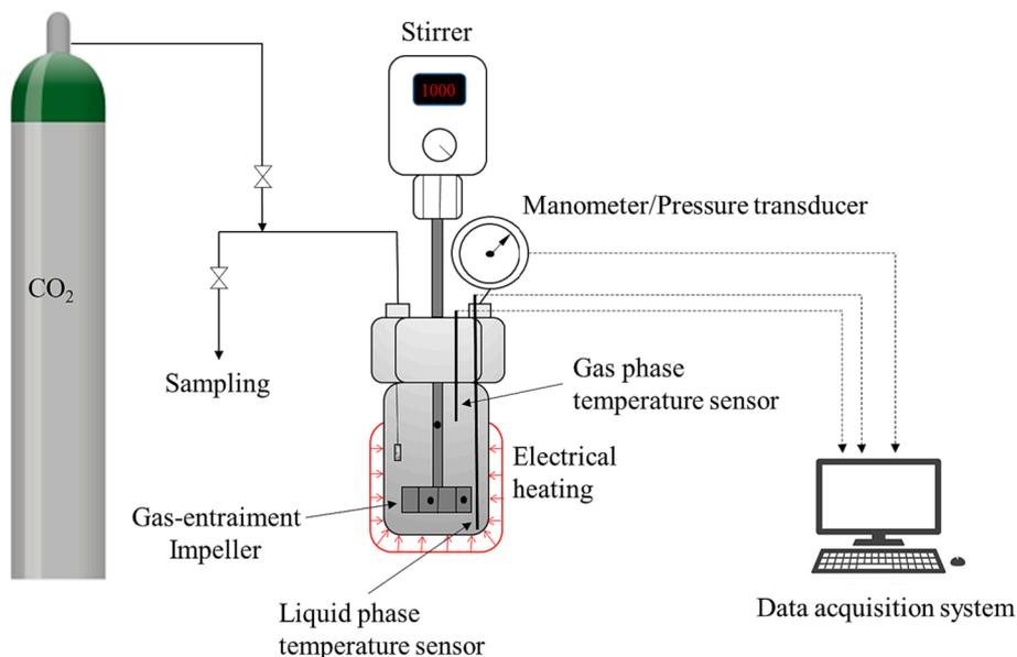
**Fig. 3.** Schematic view of the carbonation reactor system.
