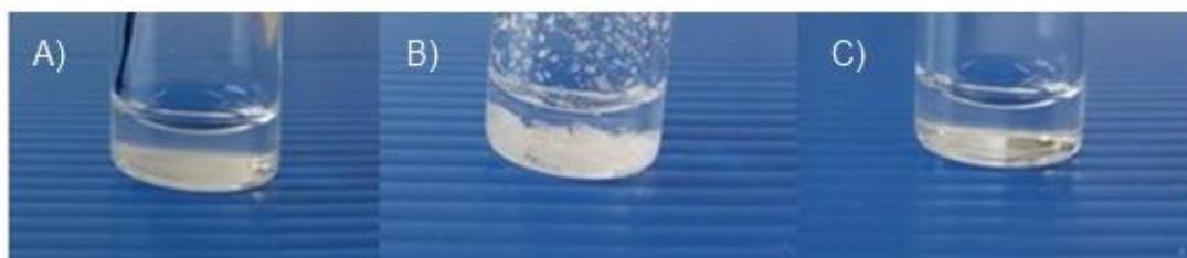
Figure 9. A) n\text{-Bu}_4\text{NCl} mixed with 1-pentyne, B) n\text{-Bu}_4\text{NCl} mixed with n -pentane, and C) n\text{-Bu}_4\text{NBF}_4 mixed with 1-pentyne, room temperature.
