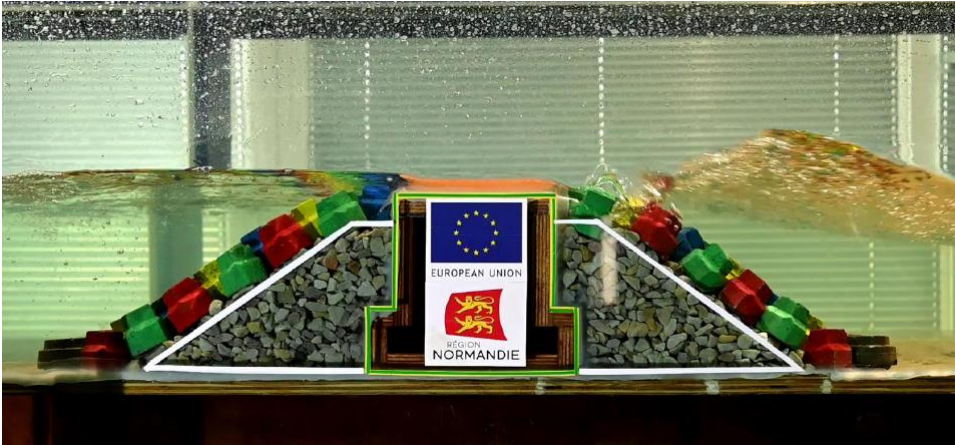
Figure 7 2D tests for Cherbourg pilot site (ESITC wave flume)
