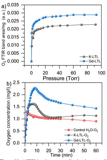
**Figure 10. a)** FTIR band area normalized to the mass of K-LTL and Gd-LTL nanosized zeolites as a function of O<sub>2</sub> pressures and b) time-dependent changes of oxygen concentration in PBS solution with addition of oxygen-saturated K-LTL and Gd-LTL nanosized zeolites and the control sample (oxygen-saturated water).
