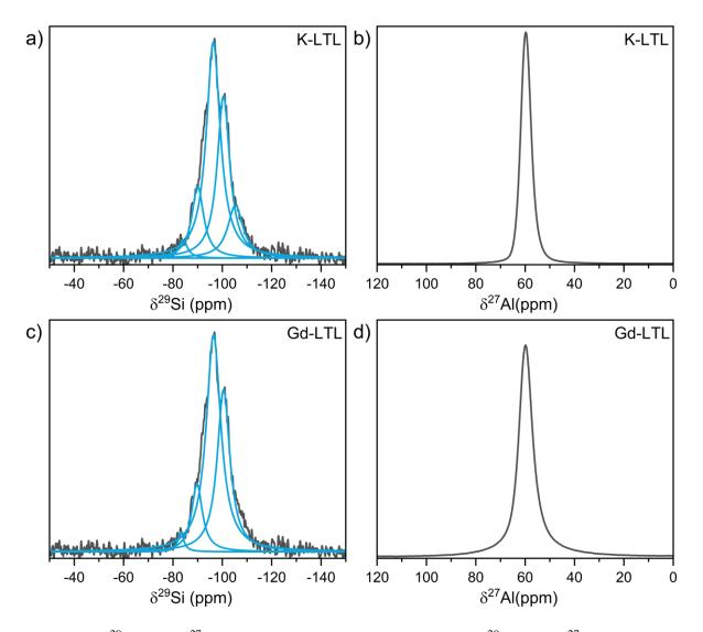
**Figure 6:** a) <sup>29</sup>Si and b) <sup>27</sup>Al MAS NMR spectra of K-LTL and c) <sup>29</sup>Si and d) <sup>27</sup>Al MAS NMR spectra of the Gd-LTL nanosized zeolites.
