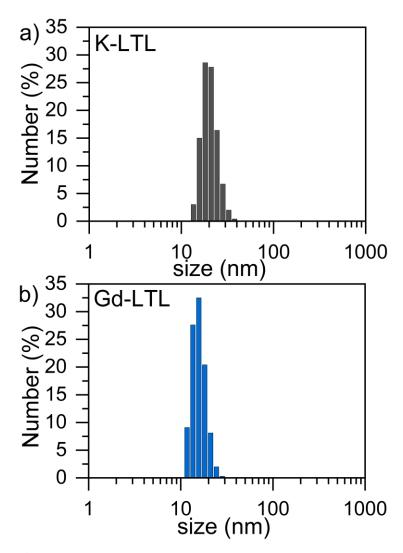
Figure 3. Dynamic light scattering profile of a) K-LTL and b) Gd-LTL nanosized zeolites.
