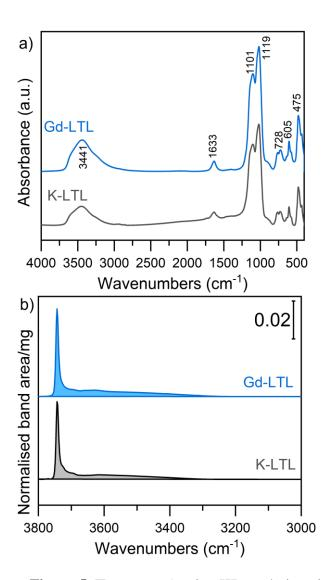
**Figure 5.** IR spectra a) using KBr technique in the range 400-4000 cm<sup>-1</sup> and b) using self-supported pallet in the range 3000-3800 cm<sup>-1</sup> of K-LTL and Gd-LTL nanosized zeolites
