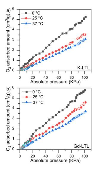
**Figure 9.** Oxygen adsorption isotherms of a) K-LTL and b) Gd-LTL nanosized zeolites at different temperatures
