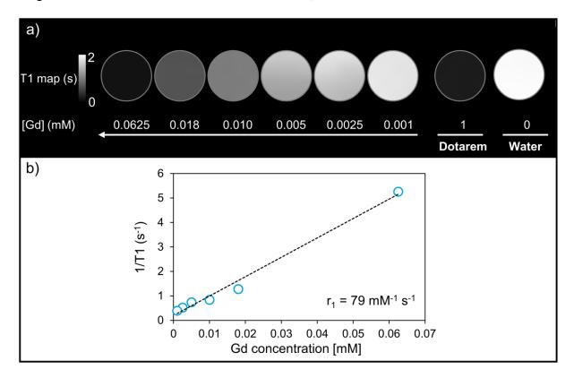
**Figure 11.** a) T1 map MR images as a function of Gd(III) ion concentration and b) Plots of the R1 value (1/T1) as a function of Gd(III) ion concentration. Slope provide r1 value
