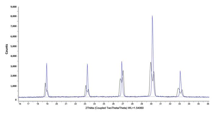
**Figure 12.** 50% mass after Spray drying protocol 2: (black pattern) solid collected in the upper part of the drying chamber; (blue pattern): solid from the collector bowl.
