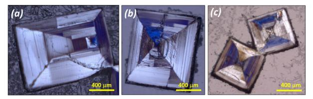
**Figure 4.** Polarized-light optical microscopy (POM) of selected NaClO<sub>3(x)</sub>BrO<sub>3(1-x)</sub> mixed crystals grown by complete evaporation at 20 °C from 50 wt.% NaClO<sub>3</sub>/NaBrO<sub>3</sub> mixtures in aqueous solution. (**a**–**c**) show single crystals revealing domains of different handedness. Hopper defects (concave crystals) were often found because crystal edges and corners grow faster than surfaces for large crystals grown at high supersaturation without stirring.
