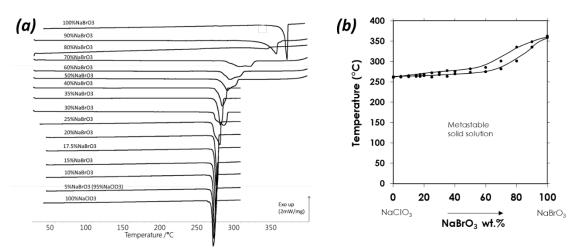
**Figure 11.** (a) DSC analyses (heating rate 5 K.min<sup>-1</sup>) of powder samples prepared by spraydrying (Protocol 1). (b) Racemic binary section of the quaternary system:  $(NaClO_3)_L/(NaClO_3)_D/(NaBrO_3)_L/(NaBrO_3)_D$ . for which a metastable solid solution could be obtained.
