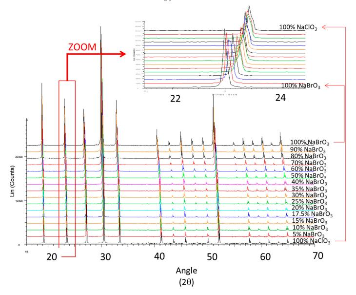
**Figure 9.** XRPD pattern versus composition of NaClO<sub>3(x)</sub>BrO<sub>3(1-x)</sub> (mass fraction) prepared by spray-drying-protocol 1-The inlet is a zoom on the second peak at ca. 23 ° (2 $\theta$  scale Cu K $\alpha$ ).
