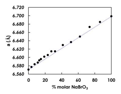
**Figure 10.** Crystallographic parameter **a** of the complete metastable solid solution  $NaClO_{3(x)}BrO_{3(1-x)}$  (molar fraction) prepared by spray-drying -using protocol 1 (precise values are reported in Table S1). A deviation from the Vegard law (apparent non-linearity) seems present for some compositions. The blue line is for guiding the eyes.
