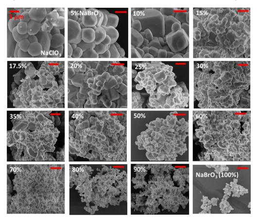
The obtained particles exhibit morphologies more isotropic than crystallization from stagnant solution for which the habitus is flattened with characteristic defects (Figure 8).
