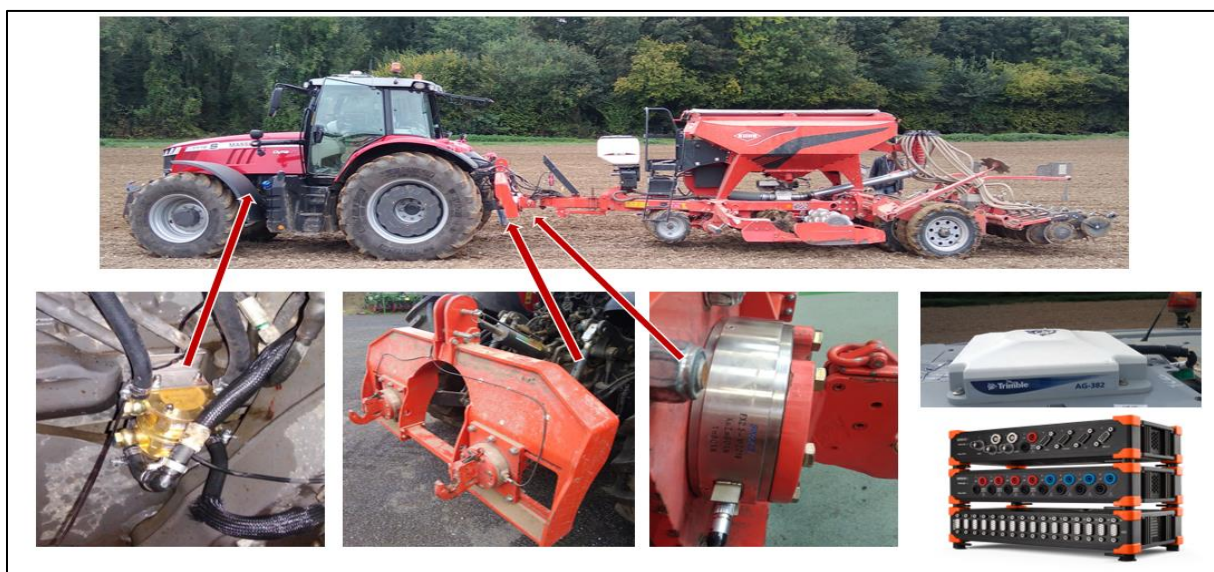
Figure 2: Energetical data acquisition setup. a. general view of the tractor-seeder assembly. b. volumetric differential flow meter, c. dynamometric frame, d. three-axial force transducer, e. GPS-RTK receiver, f. universal acquisition unit.
