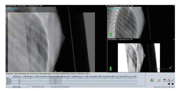
Figure 1 Screen capture of the repositioning imaging performed on a Clinac 2100<sup>®</sup>, by double exposure for a patient irradiated on the left breast. The left part of the screen shows the matching obtained between the daily imaging and the reference one (digitally reconstructed radiograms, DRR), the right window shows the DRR (top) and the daily image (bottom). In the lower strip of the window are displayed the corrections to apply and the status of medical approval.
