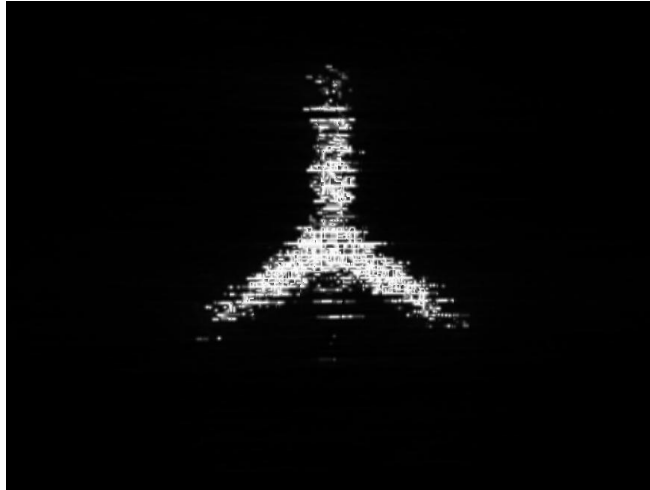
Fig. 11. 3D shape visualization of the Y particle created from 120 angles of view (see visualization 4)
