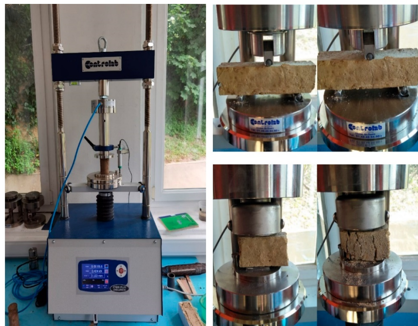
Figure 6. Press-machine (left), flexural test (right top), and compression test (right bottom).
