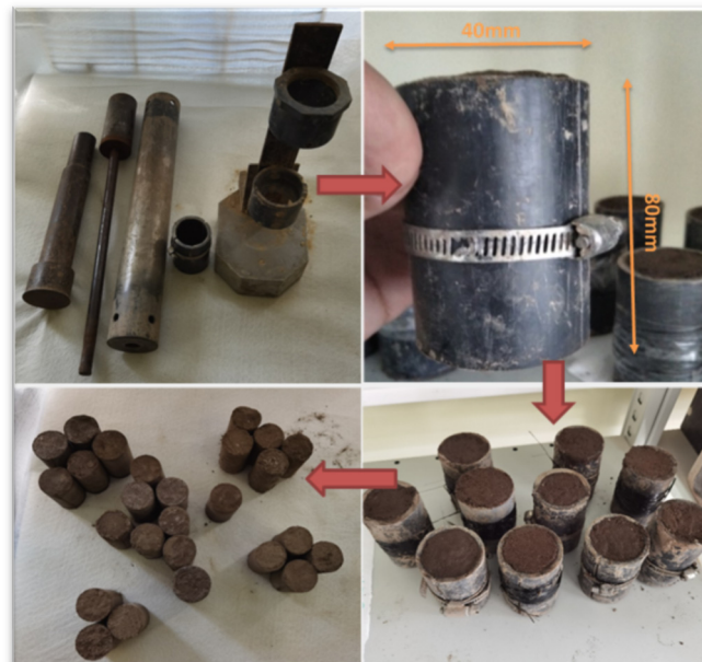
Figure 7. Sample preparation by compacting them at normal Proctor energy.
