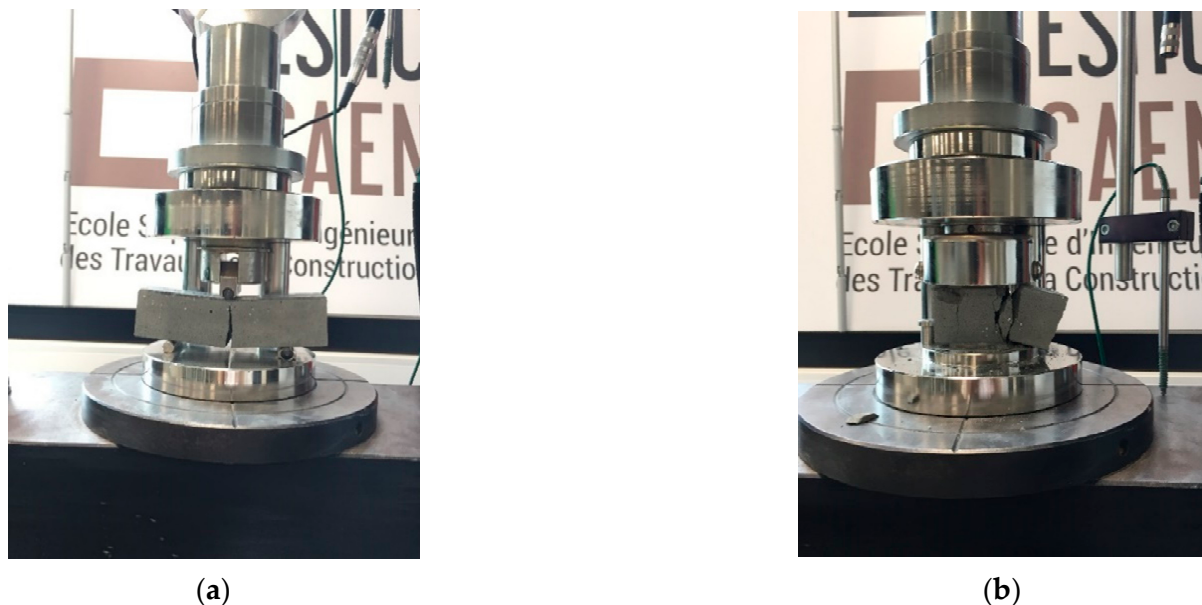
Figure 5. Mechanical test equipment. (a) Flexural three-point test. (b) Compression test.
