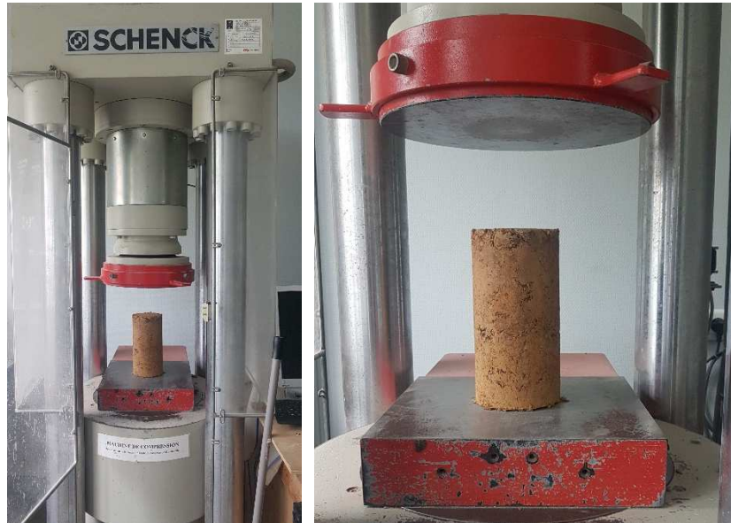
Figure 5: Cob sample to be tested under the INSTRON SCHENCK press.
