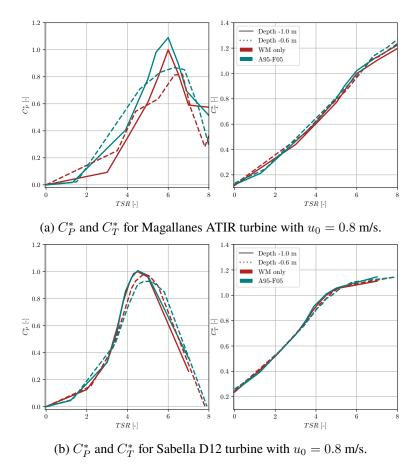
FIGURE 5 – Performances of ATIR and D12 turbines versus TSR.
