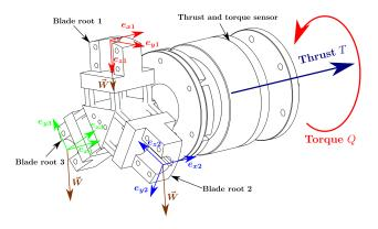
FIGURE 3 – Axis system for each blade root load and represention of weight  $\vec{W}$  for each blade. The weight is represented at the center of the axis system, and not at the gravity centre, to ease representation.
