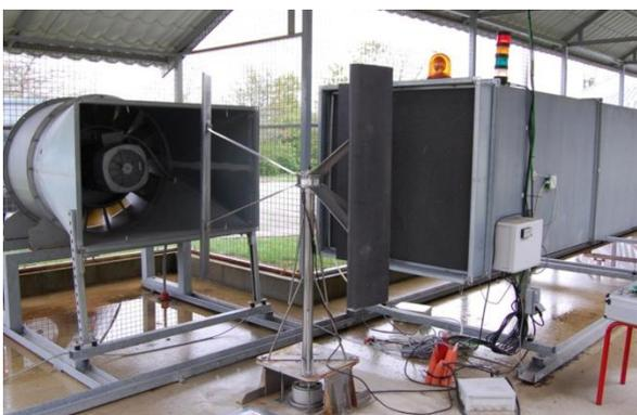
Fig 2. Experimental wind tunnel
