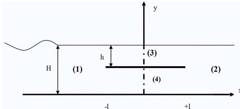
Fig. 2: Configuration of plate submerged breakwater.
