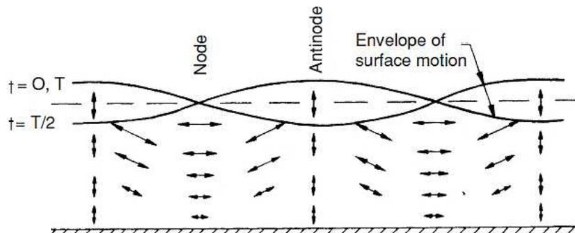
Fig. 6: Standing wave and surface profile envelope.
