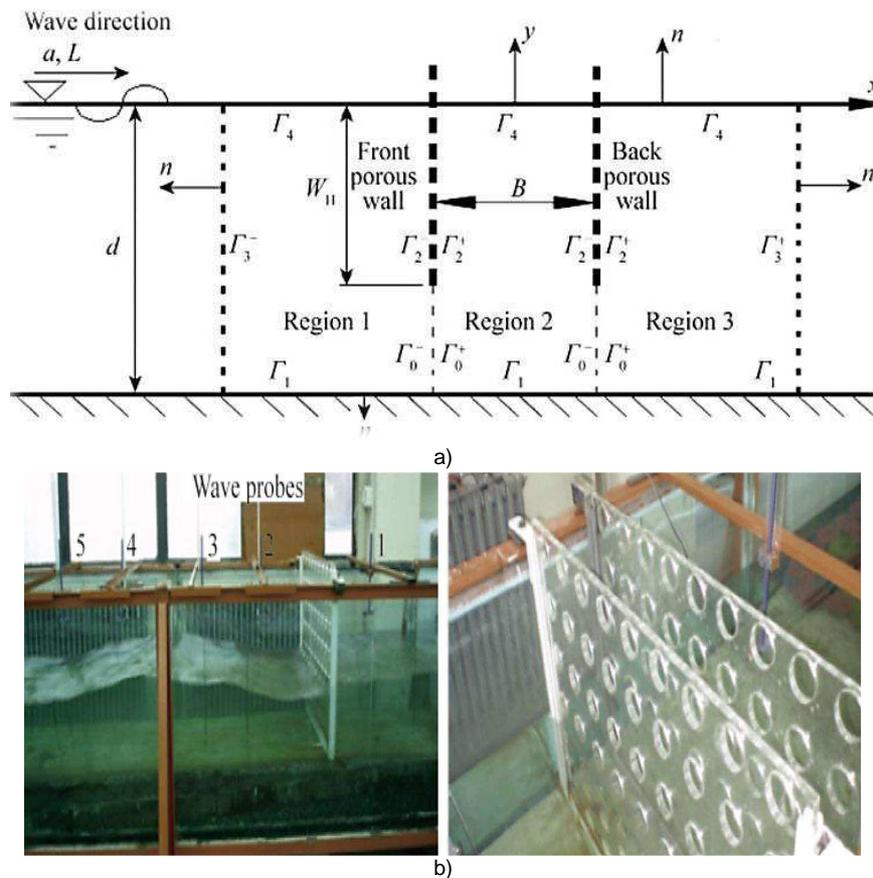
Fig. 3: Perforated breakwater: a) scheme, b) experiment [38].
