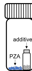
Figure 2. Schematic of the sample environment for the preparation of \gamma form crystals in the presence of additives
