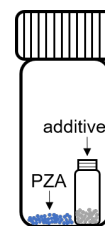
Figure 2. Schematic of the sample environment for the preparation of \gamma form crystals in the presence of additives
