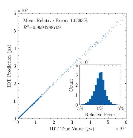
Figure 9: Comparison between the IDT reference true values and the predictions by the basic ANN on the test set. The subplot shows the distribution of relative errors.
