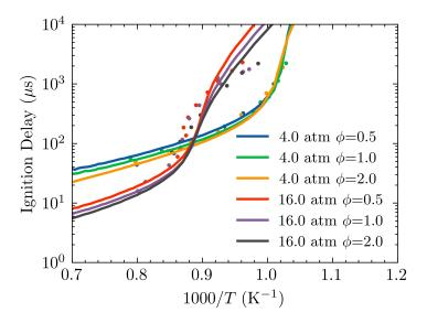
Figure 5: Comparisons between the HyChem simulated (lines) and experimental measured (symbols) IDTs of hydrogen under various temperature, pressure and equivalence ratio conditions.
