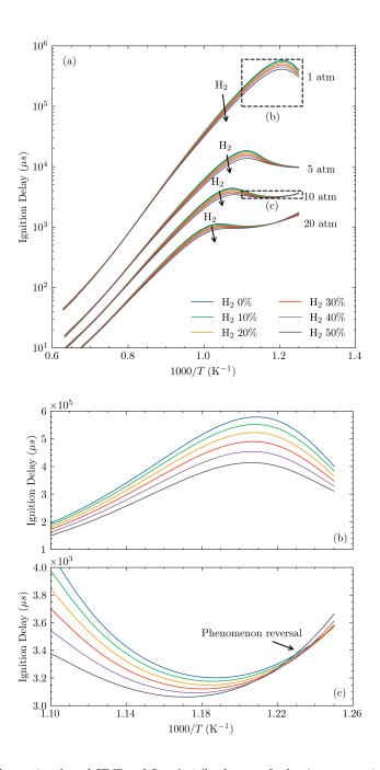
Figure 6: HyChem simulated IDTs of Jet A-1/hydrogen fuel mixture at  $\phi = 1.0$ . (a) The blending molar ratio of hydrogen increases in the arrow direction for each pressure group profiles; (b) Zoomed-in profiles for P = 1 atm; (c) Zoomed-in profiles for P = 10 atm.
