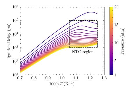
Figure 8: HyChem simulated IDTs of Jet A-1/hydrogen fuel mixture at  $\phi = 1.0$  and R = 50%. The pressure between 1 atm and 20 atm is indicated by the color of the curves.
