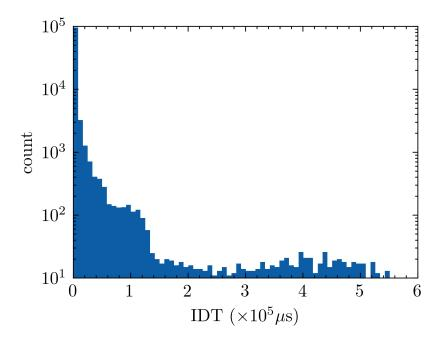
Figure 1: Long tail distribution of IDT (ignition delay time) values of Jet A-1/hydrogen fuel mixture in the obtained database containing 104,000 samples.
