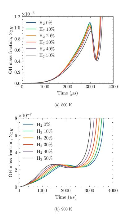
Figure 7: Time evolution of OH mass fraction during the ignition process of Jet A-1/hydrogen fuel mixture at P=10 atm and  $\phi=1.0$ .
