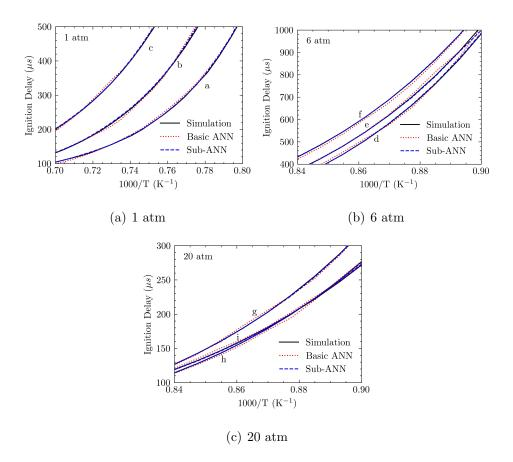
Figure 12: Comparison of the IDT profiles predicted by HyChem simulation, the basic ANN and the nested sub-ANN approach. 9 typical cases are plotted. Case a:  $\phi=0.5, R=0\%$ . Case b:  $\phi=1.0, R=20\%$ . Case c:  $\phi=1.5, R=40\%$ . Case d:  $\phi=0.5, R=0\%$ . Case e:  $\phi=1.0, R=20\%$ . Case f:  $\phi=1.5, R=40\%$ . Case g:  $\phi=0.5, R=0\%$ . Case h:  $\phi=1.0, R=20\%$ . Case i:  $\phi=1.5, R=40\%$ .
