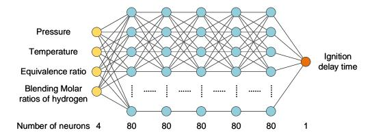
Figure 2: Structure of the basic ANN model. 4 input features: pressure, temperature, equivalence ratio and blending molar ratio of hydrogen. 5 hidden layers with 80 neurons in each one. Output layer: IDT.
