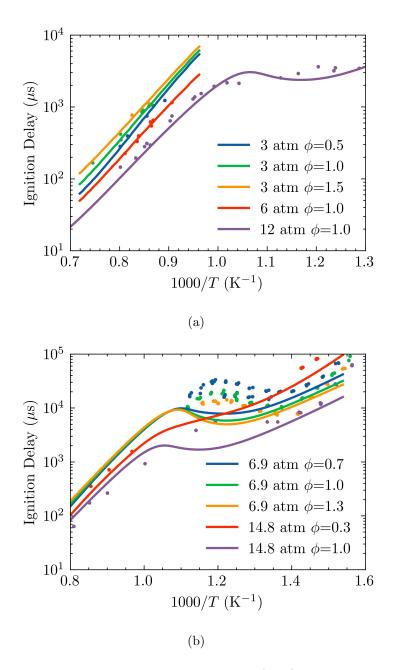
Figure 4: Comparisons between the HyChem simulated (lines) and experimental measured (symbols) IDTs of Jet A-1 under various temperature, pressure and equivalence ratio conditions.
