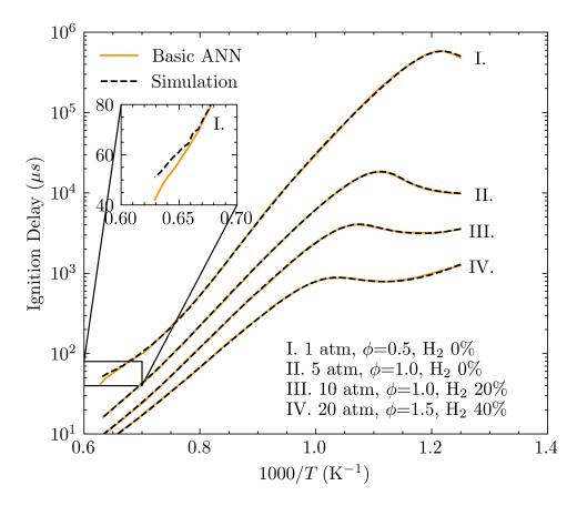
Figure 10: Comparison between the HyChem simulated IDT profiles and the basic ANN predictions under various pressure, equivalence ratio and hydrogen blending ratio conditions. The subplot is the zoomed-in view of the Case I.
