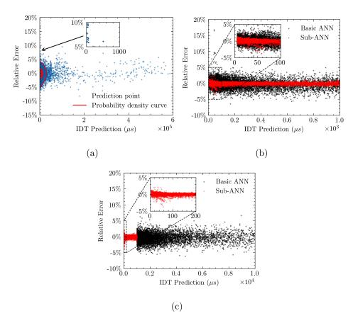
Figure 11: Scatter plots of relative errors against IDT predictions by the ANN models. (a) Results of the basic ANN model. (b) Comparison between the basic ANN and the sub-ANN for IDT  $< 10^3$  µs. (c) Results of the combined dual-ANN model.
