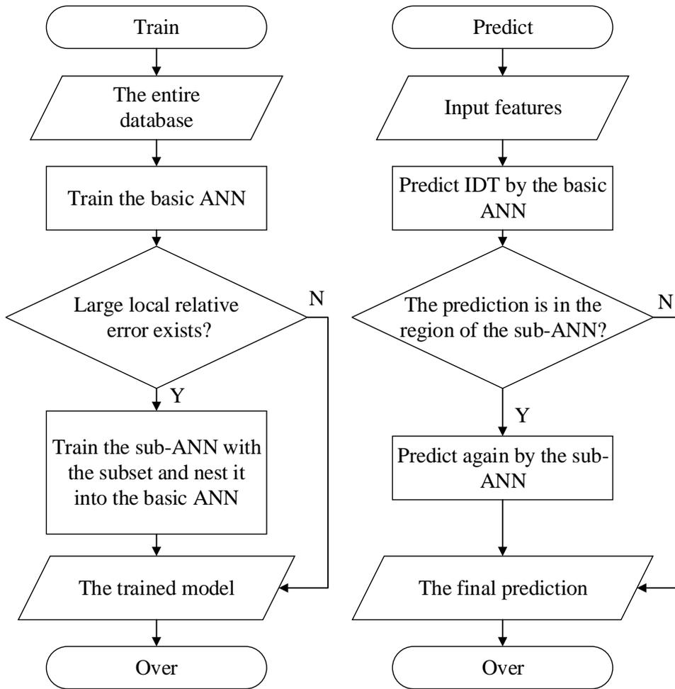
Figure 3: Flowchart of the overall training (left) and predicting (right) processes of the nested sub-ANN approach.
