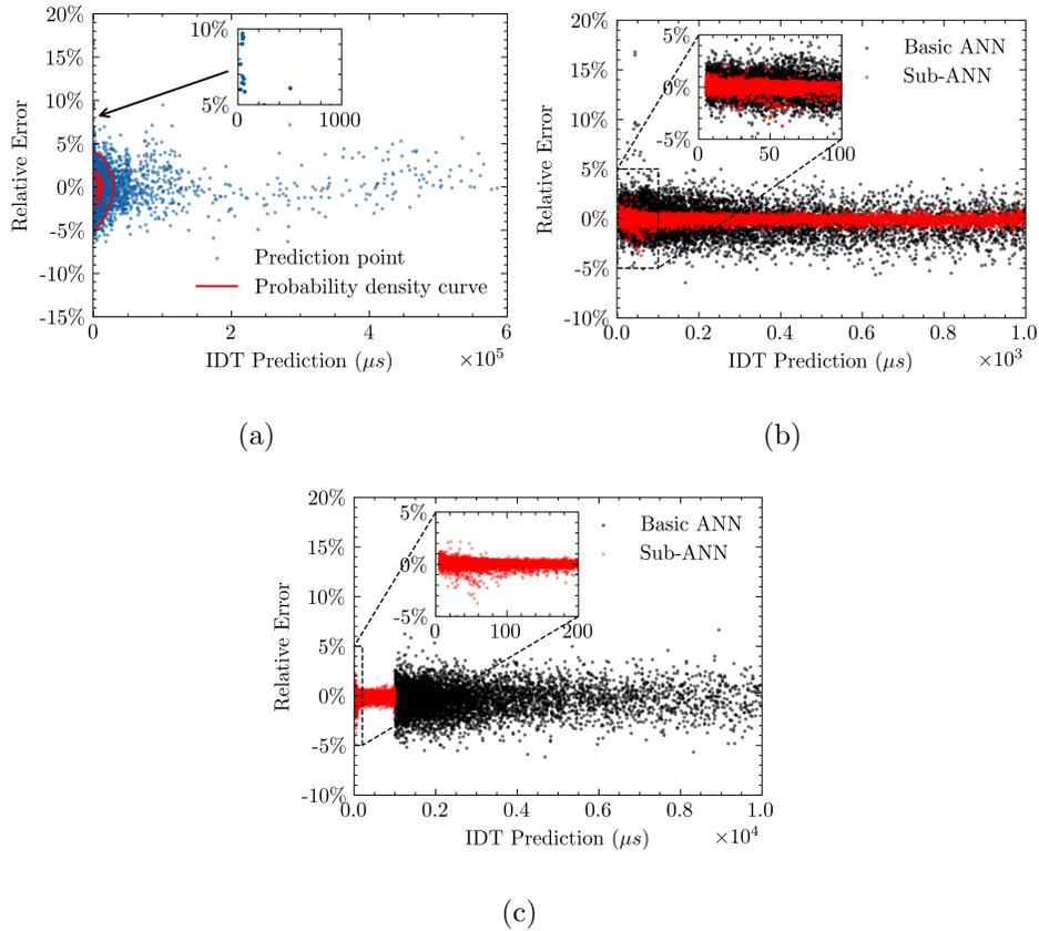
Figure 11: Scatter plots of relative errors against IDT predictions by the ANN models. (a) Results of the basic ANN model. (b) Comparison between the basic ANN and the sub-ANN for IDT <  $10^3 \mu s$ . (c) Results of the combined dual-ANN model.
