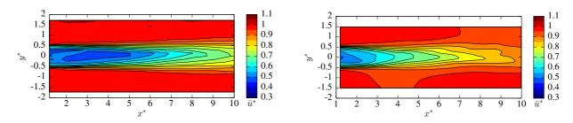
Figure 8. Wake velocity comparison with the experimental velocity maps of Mycek et al. [22]. Left is the experimental and right is the numerical velocity map for TSR = 3.67,  $I_{\infty} = 3\%$  and  $\lambda = (0.1, 0.1, 0.1)$ .
