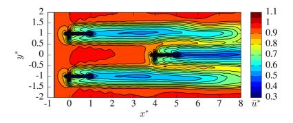
Figure 3. Post-treated velocity map of 3 interacting turbines immersed in incoming flow. Here, the ambient turbulence intensity is set to  $I_{\infty} = 0\%$ . The image is reproduced from Mycek *et al.* [24].
