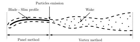
Figure 1. Scheme describing the different methods used in the software. The blade is supposed infinitely thin and is presented as cutsection.
