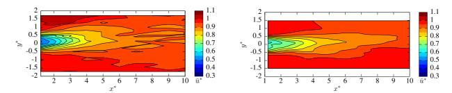
Figure 9. Wake velocity comparison with the experimental velocity maps of Mycek *et al.* [22]. Left is the experimental and right is the numerical velocity map for TSR = 3.67,  $I_{\infty} = 15\%$  and  $\lambda = (0.1, 0.1, 0.1)$ .
