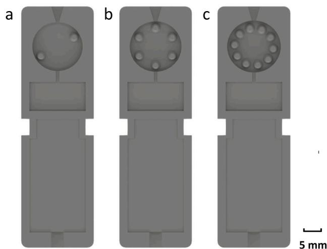
**Fig. 1.** The three mould designs used in this study. a) 2 Pin b) 6 Pin c) 10 Pin.
