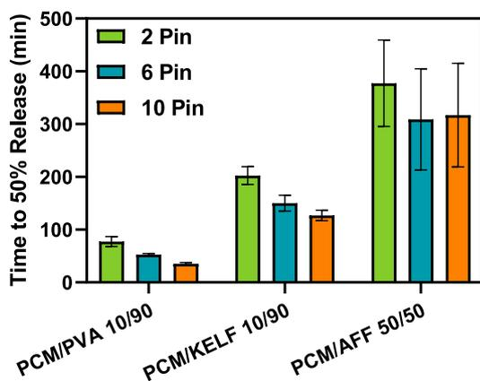
Fig. 11. The time taken for formulations to reach 50% drug release for each formulation split by tablet geometry.
