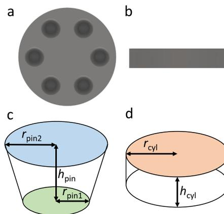
**Fig. 2.** Schematic of tablet design features. a) A top and b) side view of a tablet produced from the 6 Pin design; c) design of an individual pin; d) design of the basic cylindrical tablet structure.
