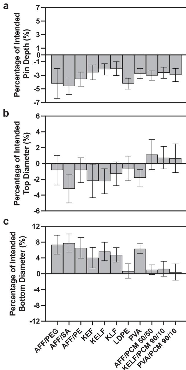
Fig. 5. Tablet pin characteristics measured by OCT. a) The depth of the pins on the tablet surface ( $h_{pin}$  from Fig. 2c) b) The top surface diameter of the pins on the tablet surface ( $2 \times r_{pin1}$  from Fig. 2c) c) The bottom surface diameter of the pins on the tablet surface ( $2 \times r_{pin2}$  from Fig. 2c) a-c: for each bar  $n = 6$  measurements with the error bars representing the standard deviation.
