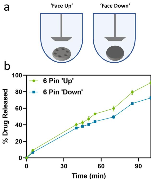
Fig. 9. Impact of anisotropic tablet structure on drug release profiles of the PVA/PCM 90/10 formulation. a) A depiction of the 'Face Up' and 'Face Down' orientation that tablets may adopt in the dissolution vessels b) 6 Pin PVA/PCM 90/10 tablets split by 'Face up' and 'Face down'. Sample size for 'Face up' is 4 tablets and for 'Face down' is 2 tablets. Error bars represent the 95% confidence intervals.
