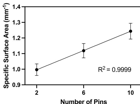
Fig. 10. The average specific surface area for all formulations vs. the number of pins in the tablet geometry. Error bars represent the standard deviation.
