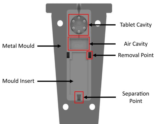
Fig. 3. The mould insert for the 6 Pin Design inserted into the metal mould. This depiction represents one half of the full mould.
