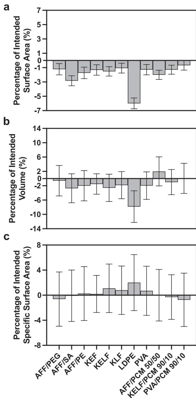
Fig. 7. Analysis of the actual surface area, volume and specific surface area compared to the digital design. a) The average surface area for each formulation as calculated by Eq. 1. b) The average volume for each formulation as calculated by Eq. 2. c) The average specific surface area for each formulation as calculated by Eq. 3. a-c: for each bar,  $n = 60$  tablets for LDPE and  $n = 18$  for all other formulations with the error bars representing the propagated standard deviation.
