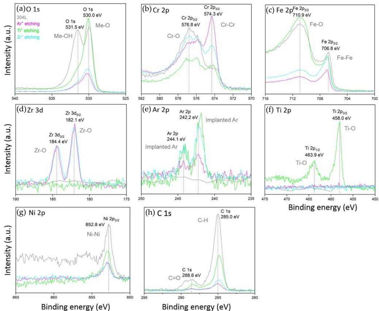
**Figure 3.** High-resolution XPS spectra of (a) O 1s, (b) Cr 2p<sub>3/2</sub>, (c) Fe 2p<sub>3/2</sub>, (d) Zr 3d, (e) Ar 2p, (f) Ti 2p, (g) Ni 2p and (h) C 1s of raw and etched 304L samples.
