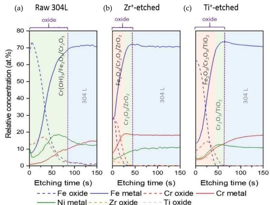
**Figure 4.** XPS depth profiles of (a) raw 304L steel and (b) Zr<sup>+</sup>- and (c) Ti<sup>+</sup>-etched samples.
