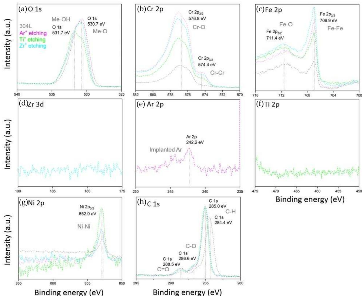
**Figure 10.** High-resolution XPS spectra of (a) O 1s, (b) Cr  $2p_{3/2}$ , (c) Fe  $2p_{3/2}$ , (d) Zr 3d, (e) Ar 2p, (f) Ti 2p, (g) Ni 2p and (h) C 1s of raw and etched 304L steel after 48 h in nitric acid solution at boiling temperature.
