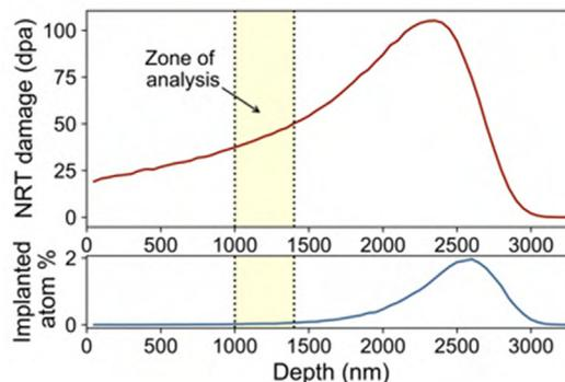
**Fig. 1.** Implantation and damage profiles from SRIM for 9 MeV  $\text{Ni}^{3+}$  ion irradiations of 304L SS.
