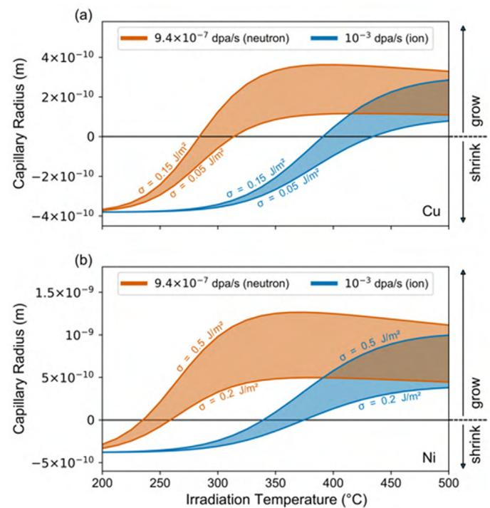
**Fig. 20.** Effective capillary radius for (a) Cu in Cu-rich clusters and (b) Ni in Ni-Si-Mn-rich clusters under irradiation as a function of temperature, calculated using the modified Heinig model.
