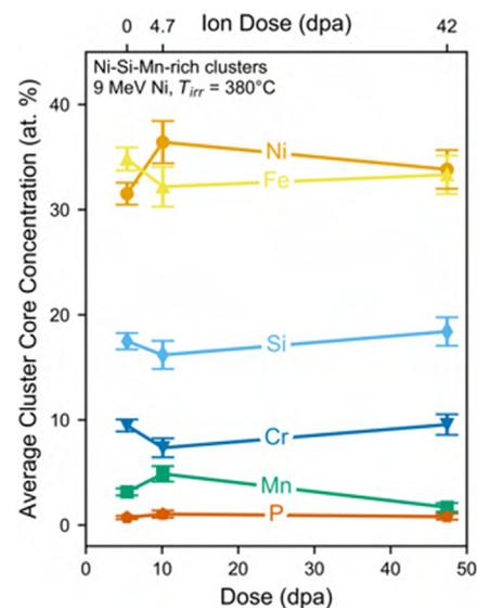
**Fig. 16.** The evolution of Ni-Si-Mn-rich cluster core composition with ion irradiation dose at 380 °C.
