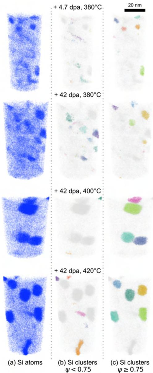
**Fig. 14.** Evolution of Si-rich clusters after ion irradiations on 5.4 dpa neutron irradiated samples. (a) Maps of Si atoms. (b) and (c) are maps showing the corresponding Si clusters identified with OSCAR for  $\psi < 0.75$  and  $\psi \geq 0.75$ , respectively. Note that other elements in the clusters are not represented here. Samples were initially irradiated in the BOR-60 reactor for 5.4 dpa. Dose and temperatures overlaid here denote the conditions used for the ion irradiations.
