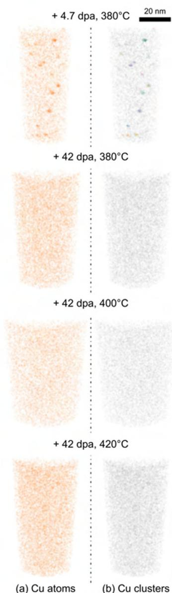
Fig. 6. Evolution of Cu-rich clusters after ion irradiations on 5.4 dpa neutron irradiated samples. (a) Maps of Cu atoms and (b) the corresponding Cu clusters identified with OSCAR. Note that other elements in the clusters are not represented here. Samples were initially irradiated in the BOR-60 reactor for 5.4 dpa. Dose and temperatures overlaid here denote the conditions used for the ion irradiations.
