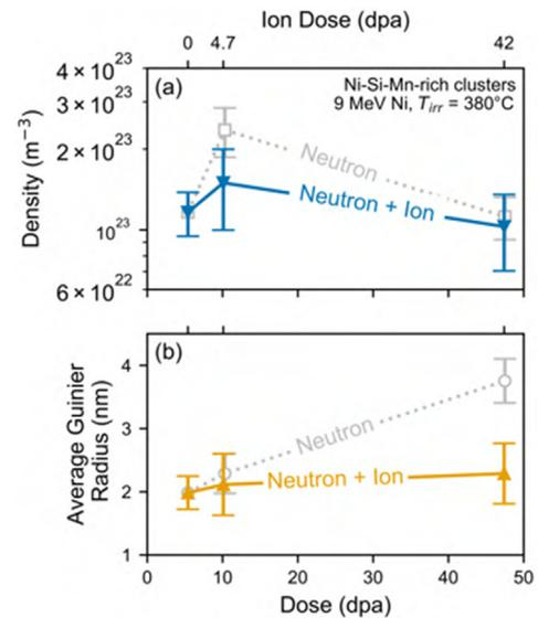
**Fig. 15.** A comparison of the (a) number density and (b) average Guinier radius of Ni-Si-Mn-rich clusters during neutron irradiation and combined neutron and ion irradiation at 380 °C.
