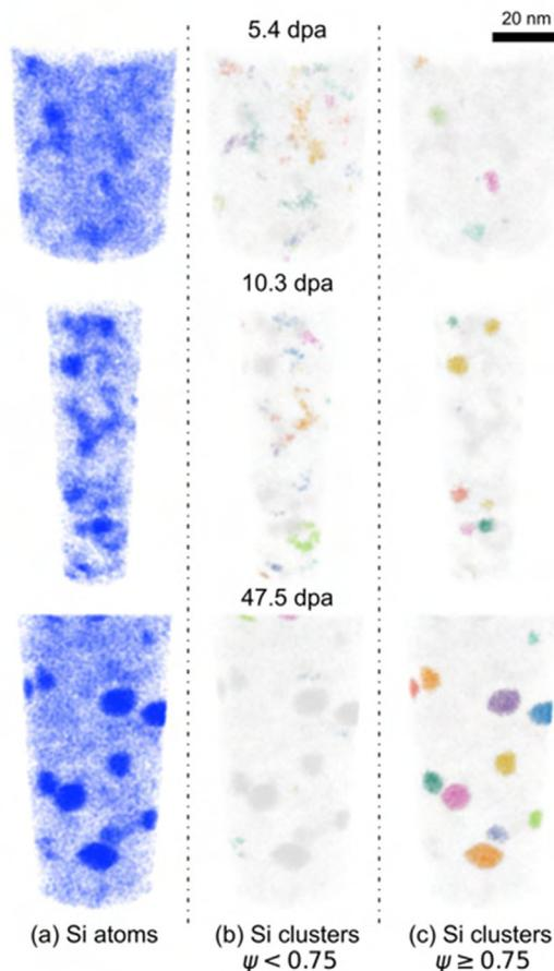
**Fig. 9.** APT reconstructions showing Si-rich clusters after fast neutron ( $E > 0.1$  MeV) irradiations in BOR-60 at 318 °C. (a) Maps of Si atoms. (b) and (c) are maps showing the corresponding Si clusters identified with OSCAR for  $\psi < 0.75$  and  $\psi \geq 0.75$ , respectively. Note that other elements in the clusters are not represented here. Neutron doses are shown above each reconstruction.
