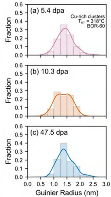
**Fig. 4.** Size distribution of Cu-rich clusters for each BOR-60 neutron irradiation dose. (a) 5.4 dpa, (b) 10.3 dpa, (c) 47.5 dpa. Kernel density estimates are plotted as solid lines.
