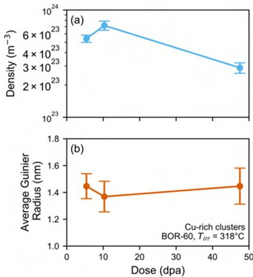
**Fig. 3.** Evolution of the number density and average Guinier radius of Cu-rich clusters with BOR-60 neutron dose for irradiations at 318 °C. (a) Number density of Cu-rich clusters as a function of neutron irradiation dose and (b) average Guinier radius of Cu-rich clusters as a function of neutron irradiation dose.
