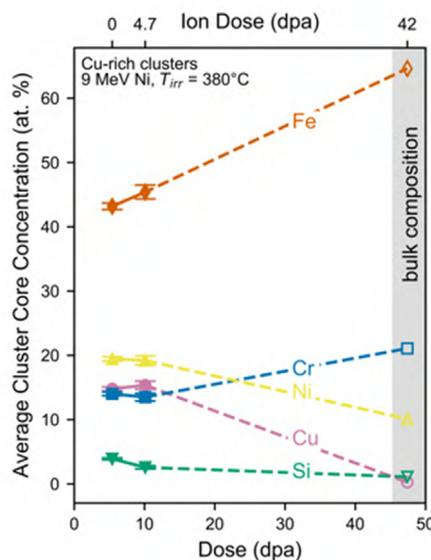
Fig. 8. The evolution of Cu-rich cluster core composition with ion irradiation dose at 380 °C. As no clusters were detected after an ion dose of 42 dpa, alloy bulk composition is plotted at this dose for reference. Dashed lines provide an interpolation of concentrations between an ion dose of 4.7 and 42 dpa.
