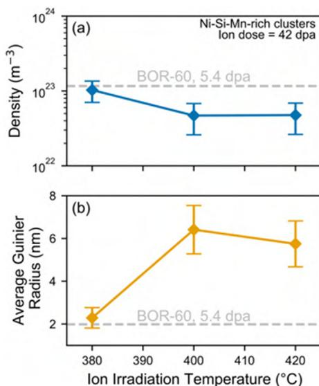
**Fig. 17.** Influence of ion irradiation temperature on (a) number density and (b) average Guinier radius for Ni-Si-Mn-rich clusters at an ion dose of 42 dpa. The cluster density and average Guinier radius for BOR-60, 5.4 dpa, which was the starting condition for ion irradiation, are indicated by the dashed lines.
