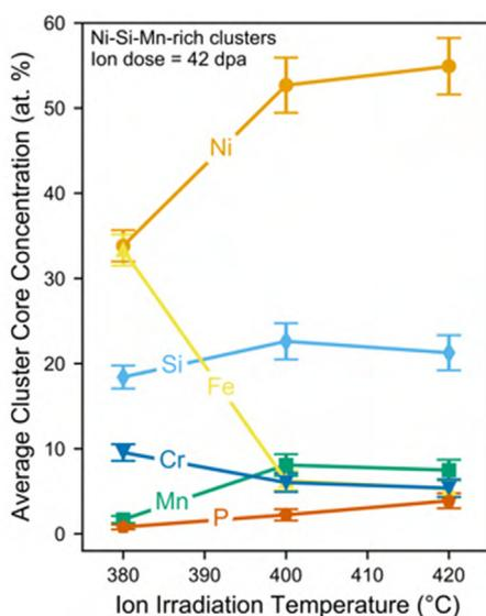
**Fig. 18.** Average core composition of Ni-Si-Mn-rich clusters as a function of irradiation temperature for an ion dose of 42 dpa.
