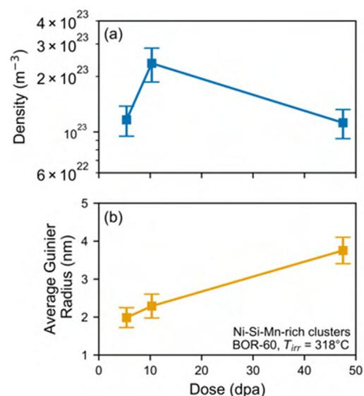
**Fig. 11.** Evolution of the number density and average Guinier radius of Ni-Si-Mn rich clusters with BOR-60 neutron dose for irradiations at 318 °C. (a) Number density of Ni-Si-Mn-rich clusters as a function of neutron irradiation dose and (b) average Guinier radius of Ni-Si-Mn rich clusters as a function of neutron irradiation dose.
