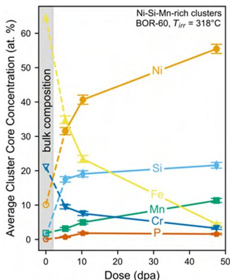
**Fig. 13.** Evolution in average core composition of Ni-Si-Mn-rich clusters with BOR-60 irradiation dose. Initial bulk composition of the alloy is shown with open symbols.
