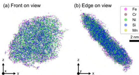
**Fig. 19.** Example of Ni-Si-rich cluster with a platelet morphology from the +42 dpa, 420 °C ion irradiation condition. (a) Front on view and (b) edge on view of the cluster. It should be noted that the cluster intersected the edge of the volume and therefore in the front on view the right-hand side of the cluster is slightly clipped.
