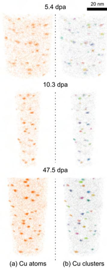
**Fig. 2.** APT reconstructions showing Cu-rich clusters after fast neutron ( $E > 0.1$  MeV) irradiations in BOR-60 at 318 °C. (a) Maps of Cu atoms and (b) the corresponding Cu clusters identified with OSCAR. Note that other elements in the clusters are not represented here. Neutron doses are shown above each reconstruction.
