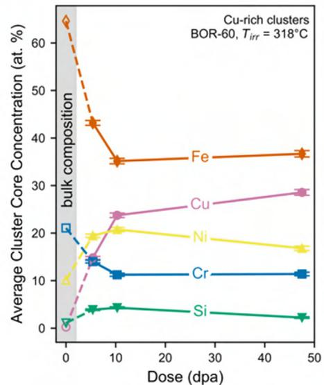
**Fig. 5.** Evolution in average core composition of Cu-rich clusters with BOR-60 neutron irradiation dose. The initial bulk matrix composition is shown with open symbols in the gray shaded area for comparison.
