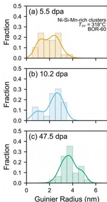
**Fig. 12.** Size distribution of Ni-Si-Mn-rich clusters for after BOR-60 neutron irradiations at 318 °C. After (a) 5.4 dpa, (b) 10.3 dpa, and (c) 47.5 dpa. Kernel density estimates are plotted as solid lines.
