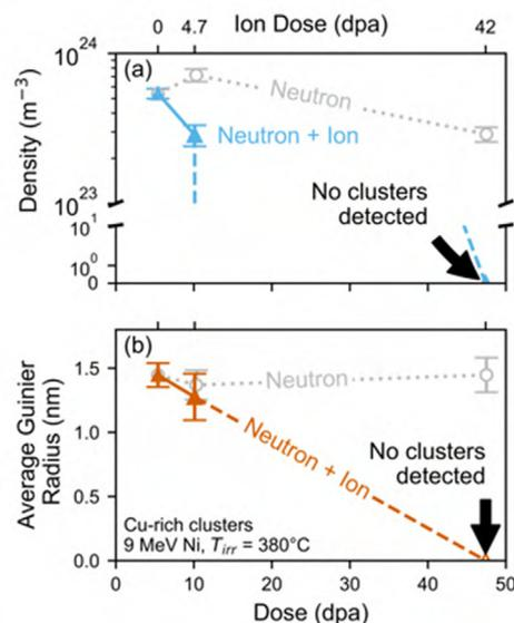
Fig. 7. A comparison of the (a) number density and (b) average Guinier radius of Cu-rich clusters during neutron irradiation and combined neutron and ion irradiation at 380 °C. Dashed lines are used to indicate that cluster number density and average Guinier radius for the combined neutron and ion irradiation are interpolated between an ion dose of 4.7 and 42 dpa as no clusters were detected at an ion dose of 42 dpa.
