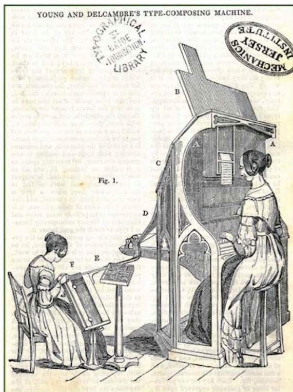
Figure 2– The Young and Delcambre composing machine. Patented 1840. Image retrieved from St Bride Library @stbridelibrary.
