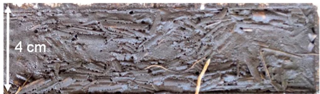
Figure 11. Fibers accumulation at the brick surface with a sieve shaker machine.
