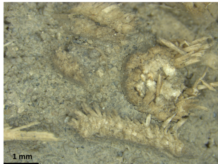
Figure 12. Microscopic image of hemp shiv inside the crude bricks.
