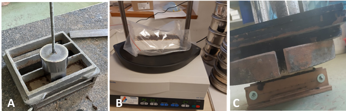
Figure 6. Bricks dynamic compaction (A), sieve shaker (B), and static compaction(C).
