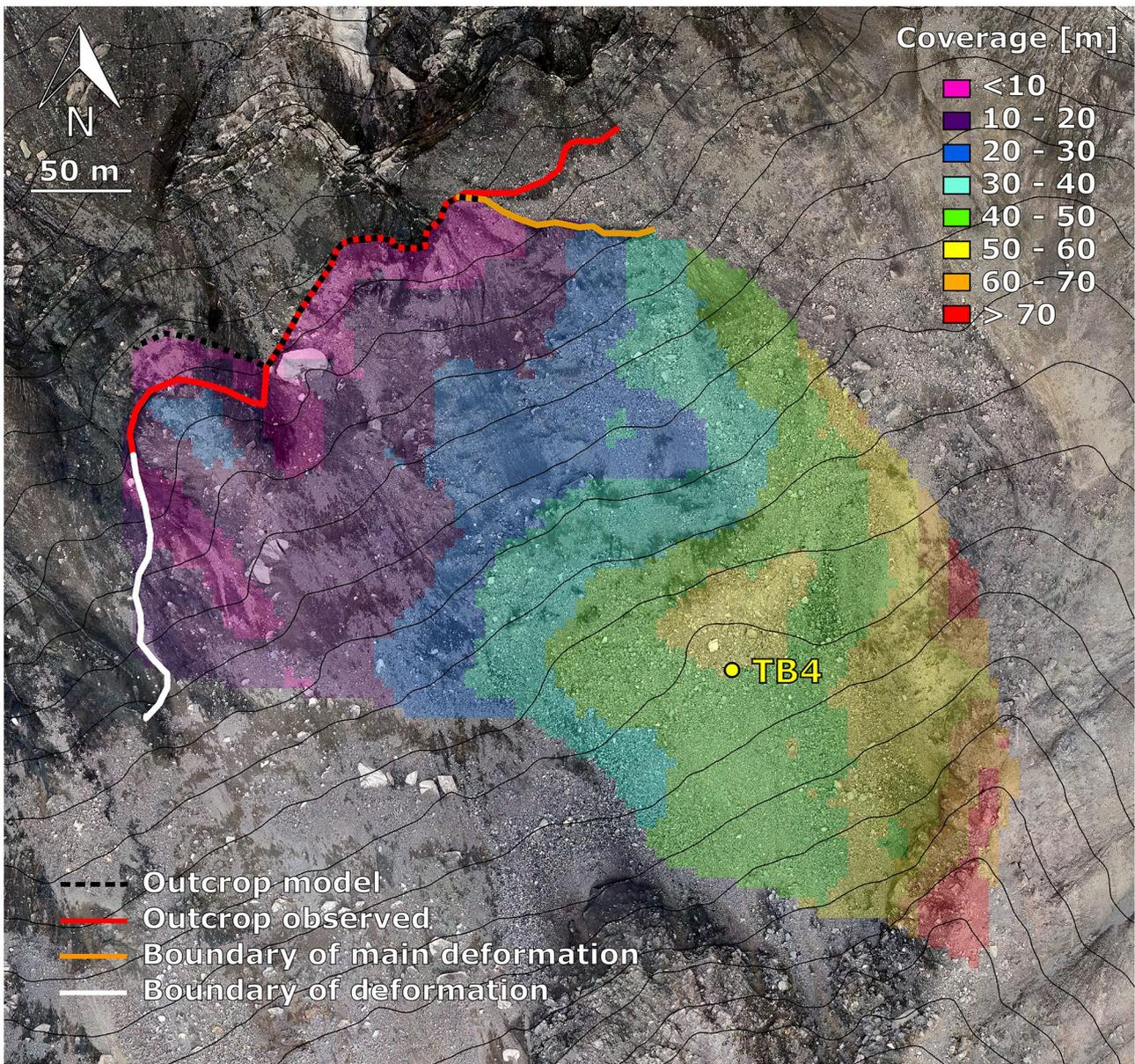
**Fig. 13** Thickness of the sliding rock mass in sector 2. The red, white, and orange lines correspond to those in Fig. 12. The black dashed line marks the intersection of the modelled sliding plane with the
