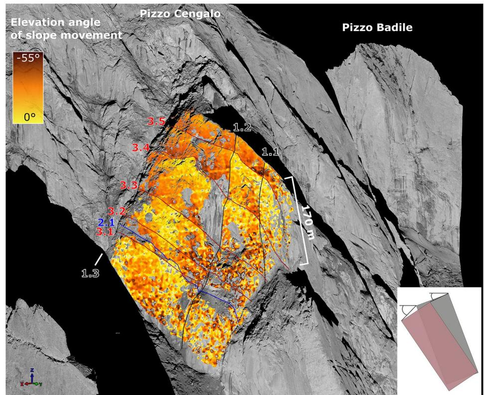
the upper edge of a joint-bordered rock body, the elevation angle is smaller and increases sharply above the outcrop lines, i.e. at the lower edge of a joint-bordered rock body. We interpret this as a toppling movement along with set 3. Set 1 delimits the toppling instability laterally, set 2 towards the back. The inset in Fig. 9 explains
