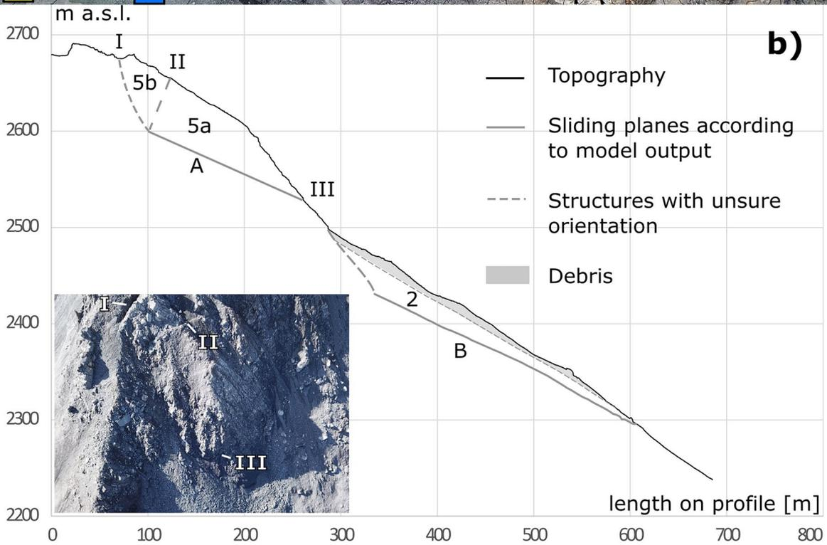
◀**Fig. 14** The colours in **a** show the elevation angle (dip) of the slope displacements, superimposed by the 2D deformation vector field in black. The red line marks the position of the slope profile in **(b)**. The profile shows the basal sliding planes A and B and is labelled with the sector names (Arabic numerals). Outcrop locations of discontinuities and sliding plane A are labelled with roman numerals. III corresponds to the outcrop line of A shown in Fig. 11a
