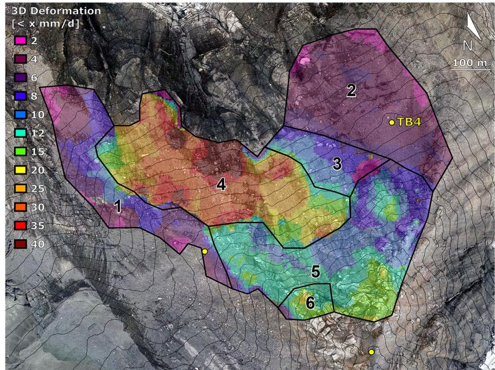
angle. Clear signs of shearing appeared along the outcrop lines of Set 3 (Figure S1). The shearing became apparent by offsets of a few cm along the joints in form of a relative heave of the rock compartment below the daylighting discontinuity and relative subsidence of the rock compartment above, similar to the pattern observed at the Brienz rock slide (Figure S2).
