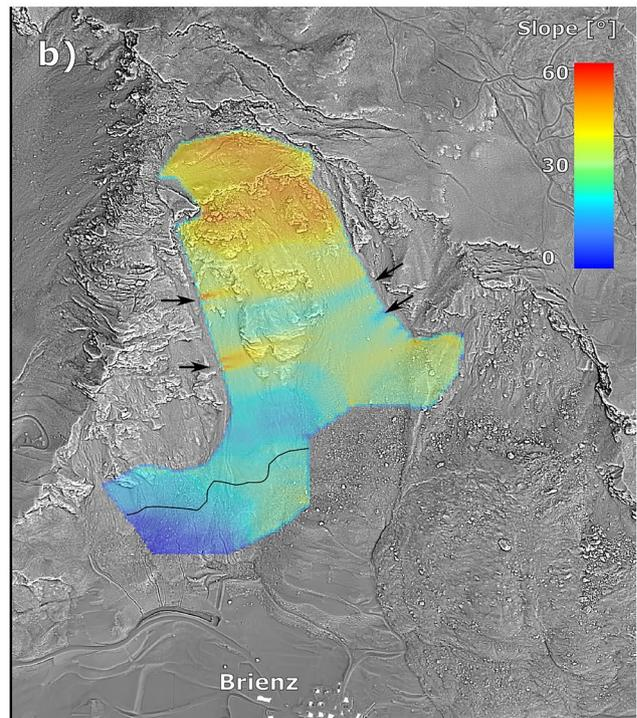
**Fig. 6** Although the elevation angle of the surface movement (a) widely corresponds to the slope of the modelled sliding plane (b), this plane crops out at the black line in part b. However, the true sliding plane likely lies at more than 100 m depth here, as indicated by borehole deformation measurements. The black arrows mark ripples
