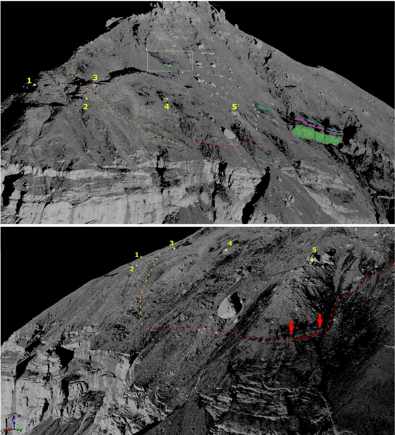
**Fig. 12** Point-cloud of the deformation area coloured by reflectivity, seen from NNE (top) and NW (bottom). The white rectangle marks the extent of Fig. 11b. The rock formations coloured in green, magenta, and blue are stable and located directly below the basal gliding plane A (sectors 1;4:5). The dashed red line marks the approximate outcrop location of gliding plane B of sector 2 in debris-covered terrain (deduced from deformation data). Red arrows mark
