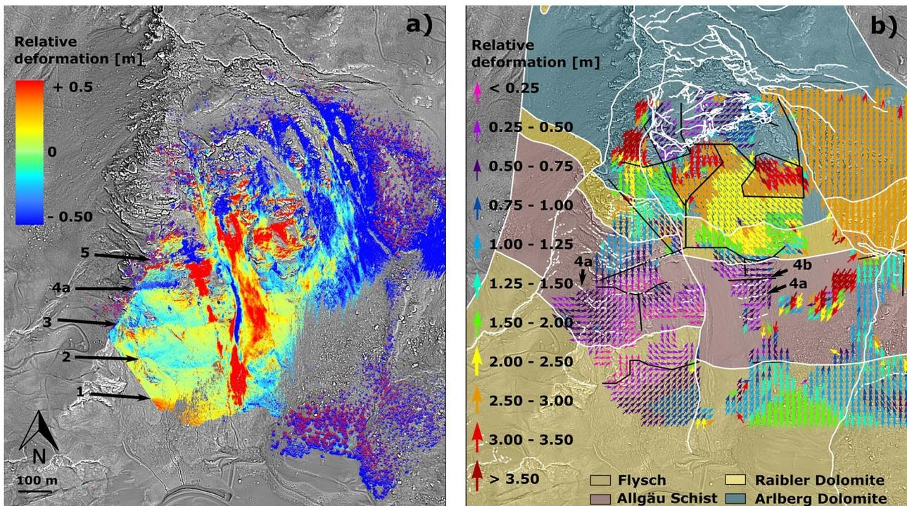
**Fig. 4** Comparison of the relative referenced point clouds from September 27, 2019, to November 30, 2020 (co-registration method B) using **a** C2M visualisation and **b** a 2D deformation vector field. The black arrows mark discontinuities at which toppling occurs. The white lineaments in part b originate from field observations and
