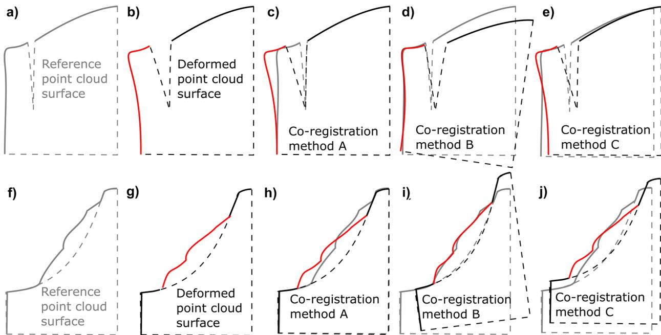
**Fig. 2** Sections through a schematic toppling (a–e) and sliding (f–j) rock slope instability, represented by point-cloud surfaces. Sketches (a) and (f) show the point cloud before, sketches (b), and (g) after
