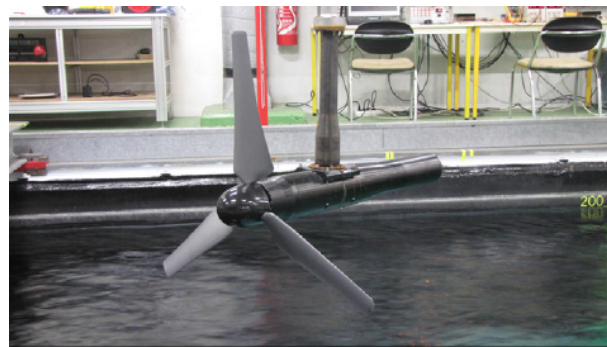
Figure 3. Tidal turbine model, Mycek et al. [6].
