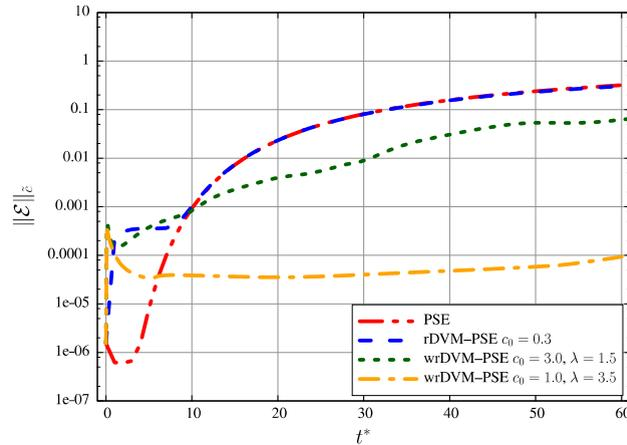
**Fig. 2.** Concentration  $L_2$  error as a function of time for the double Gaussian case. Comparison between PSE (red dashed–double-dotted line), rDVM–PSE with  $c_0 = 0.3$  (blue dashed line), wrDVM–PSE with  $c_0 = 3.0$  and  $\lambda = 1.5$  (green dotted line) and wrDVM–PSE with  $c_0 = 1.0$  and  $\lambda = 3.5$  (orange dashed–dotted line). Computations were run using a 6th order approximation and  $N = 200$  particles. Colour online.
