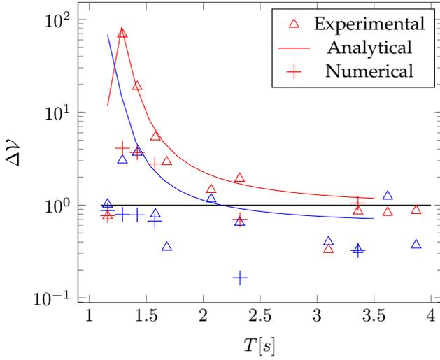
Fig. 5. Overtoppings for regular waves. Full line represents the analytical model. Red markers represent results for  $Rc/D = 0.7$  and blue for  $Rc/D = 7$ . The horizontal black line indicates the value of the overtopping ratio without buoy
