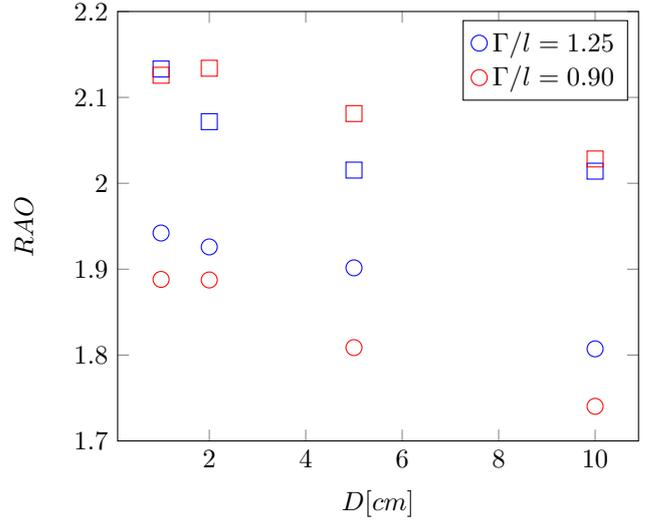
Fig. 7. Influence of the clearance distance on RAO for regular waves ( $\circ$ ) and irregular waves ( $\square$ ).
