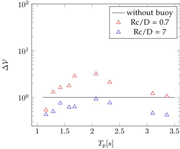
Fig. 6. Overtopping ratio measured experimentally in irregular waves.
