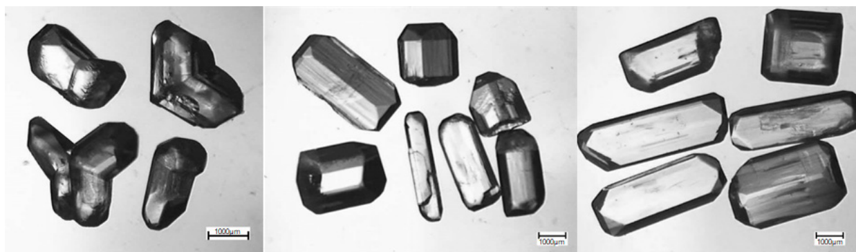
Figure 3. K_2SO_4 crystals obtained from supersaturated solutions \beta = 1.25 : typical twin crystals observed in this study (left), crystals obtained by laser irradiation (middle), and crystals obtained by spontaneous nucleation (right). Pictures were taken with a NIKON SMZ-10A microscope equipped with a Sony DXC-950 3CCD Color Video Camera Power HAD.
