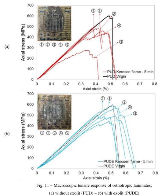
In orthotropic laminates with Exolit exposed to a kerosene flame, the preservation of tensile properties (stiffness and strength) is very good with a moderate decrease (-14%) in axial strength and an axial stiffness that is virtually unchanged in the most detrimental conditions (specimen taken from position 3). It therefore suggests that the flame-retardant additive not only delays the thermal degradation of
