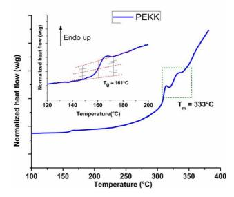
Fig. 3 – DSC curve of PEKK sample used in this study
