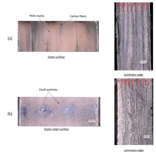
Fig. 5 – Microscopic observations of orthotropic laminates front surfaces and edges: (a) without exolit (PUD) – (b) with exolit (PUDE)
