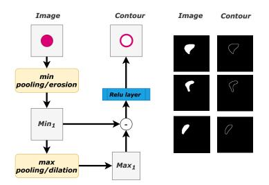
Figure 2: Principle of the contour function F: the difference (-) between the erosion (minpool) and the dilation(max-pool) layers followed by a ReLu layer. Right side: example of ground-truth segmentation image and respective contour image.
