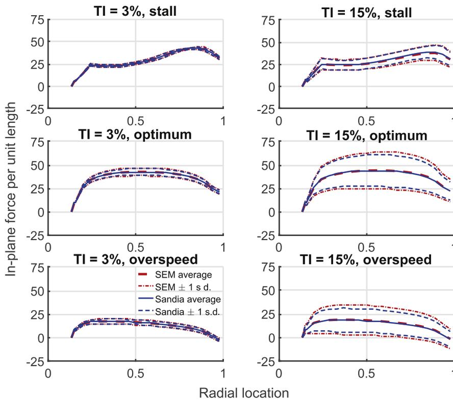
Fig. 8. Distributions of in-plane force per length on turbine blades, averaged across all blades and all runs. Average values are shown as thick lines, in red for SEM turbulence and blue for Sandia turbulence; thinner lines of corresponding colour indicate one standard deviation above and below the average. (For interpretation of the references to colour in this figure legend, the reader is referred to the Web version of this article.)
