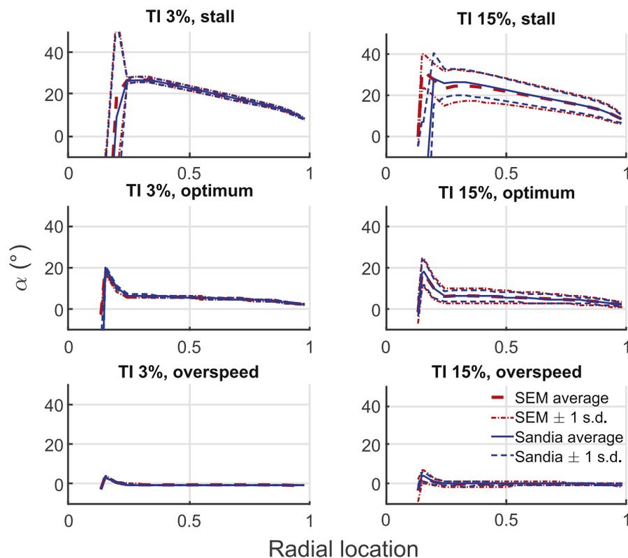
**Fig. 6.** Distributions of angle of attack on turbine blades, averaged across all blades and all runs. Average values are shown as thick lines, in red for SEM turbulence and blue for Sandia turbulence; thinner lines of corresponding colour indicate one standard deviation above and below the average. (For interpretation of the references to colour in this figure legend, the reader is referred to the Web version of this article.)
