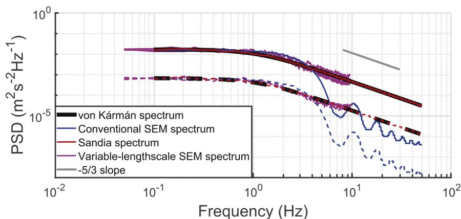
**Fig. 3.** Comparison of von Kármán spectrum and spectra from flowfields generated using the two synthetic turbulence models. Three SEM cases with variable lengthscales are shown in purple, as explained in text. Solid lines shows high-turbulence case and dashed lines show low-turbulence case. (For interpretation of the references to colour in this figure legend, the reader is referred to the Web version of this article.)
