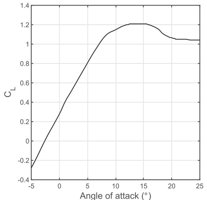
**Fig. 12.** Lift coefficient of the NACA 63418 blade section at  $Re = 6 \times 10^6$ , plotted against angle of attack for a selected range of angle of attack values encompassing stall. Data taken from Ref. [26].
