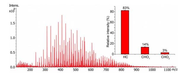
**Figure 2:** LDI (+) FTICR mass spectra of organic aerosol sample. The insert corresponds to the relative intensity of the main three molecular class observed within the sample: hydrocarbons (HC), and hydrocarbons with one (CHO<sub>1</sub>) and two (CHO<sub>2</sub>) oxygen atoms.
