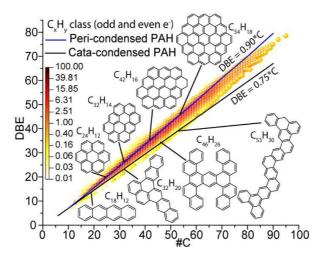
**Figure 3 :** DBE vs #C diagrams of LDI FTICR MS data from the CAST sample for hydrocarbon compounds with odd and even number of electrons. The colors indicate the relative intensity of the ions. The lower black line represents the trend of cata-condensed PAH, and the upper blue line
