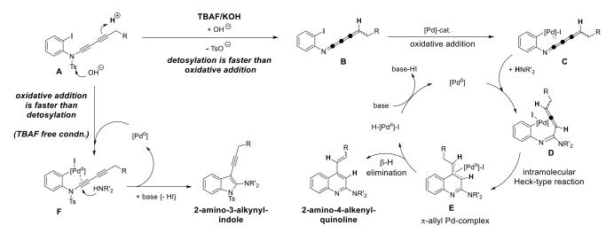
Scheme 5. Proposed mechanism for the synthesis of 2-amino-4-alkenylquinolines involving the [4]cumulenimine B and the TBAF-free pathway to 2-amino-3alkynylindoles. H atoms (bold) indicate the positions identified by deuterium incorporation experiments.
