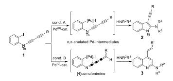
Scheme 1. Pd-catalyzed transformation of 1,3-diynamides 1 to 2-amino-3alkynylindoles 2 and its unprecedented reaction to give 2-amino-4alkenylquinolines 3 via [4]cumulenimines.
