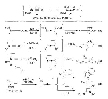
Figure 1. Resonance structures A/A' of ynamides; and ynamides as precursors of *in situ* generated ketenimine intermediates (a-d).
