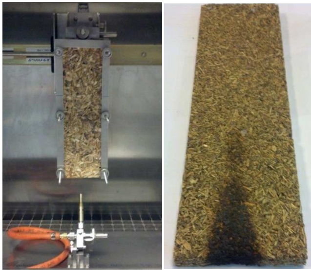
270 Fig. 4 : installation for test of resistance to fire and example of some boards after the test
