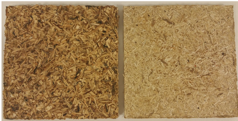
208 209 Fig. 2 : Particleboards made of big sunflower bark on the left and made of big flax shives on the right.
