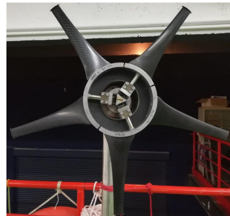
Fig. 8. Picture of the blade root load cells and the three blade supports of Sabella's D12 scaled model.
